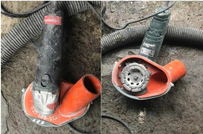
**5" angle grinder for perimeter edges with attached dust shroud. Shown 60-80 grit cup wheel on 5/8" threaded arbor**
