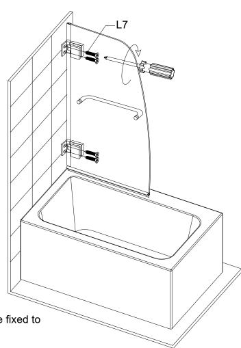
5.1、Part (L1) assembled be fixed to the wall by Part (L7).
