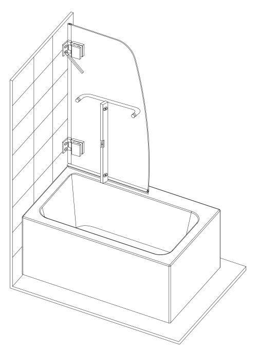
2.1、Install Part (L1) assembled against to wall and adjust position with spirit level properly. Secondly, bottom of item close to the bath. Finally, marking drill hole for hinge.
