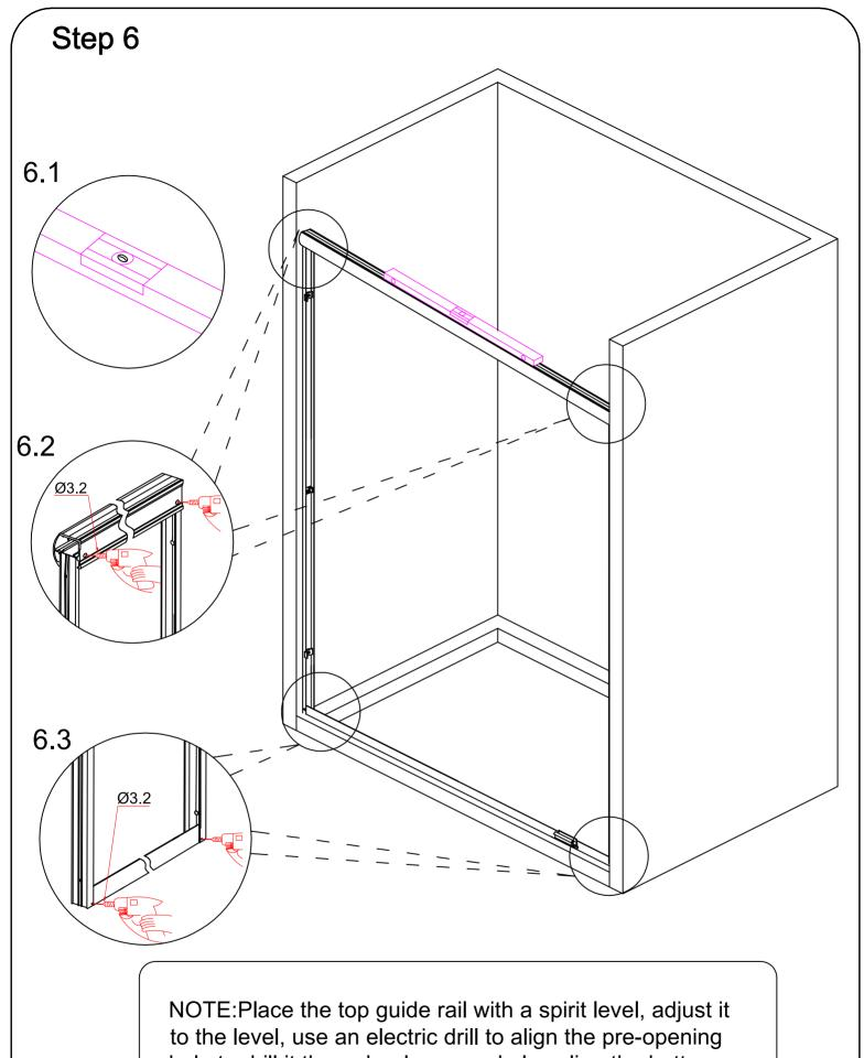
NOTE:Place the top guide rail with a spirit level, adjust it to the level, use an electric drill to align the pre-opening hole to drill it through a layer, and also align the bottom aluminum material to the pre-opened hole and drill it through a layer.
