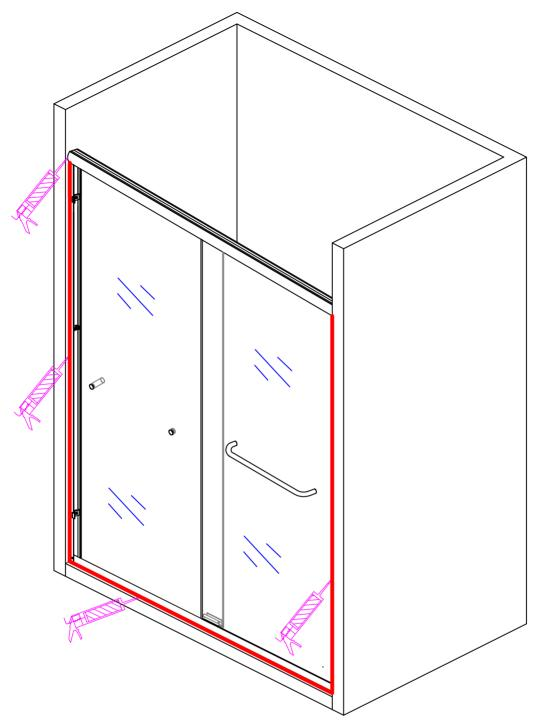
NOTE:In the last step, put glass glue on the inside of the connection between the room body, the wall and the ground, and let it stand for 24 hours before using it
