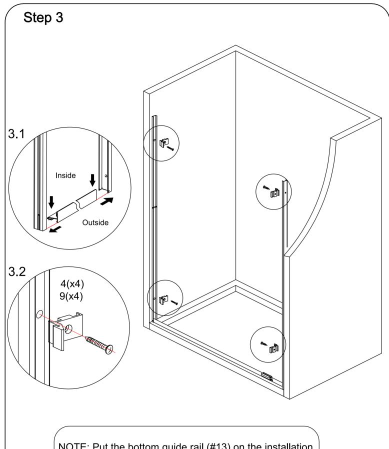
NOTE: Put the bottom guide rail (#13) on the installation position, and the wall profile (#6) fits into the bottom guide rail and presses against the wall.Install 4 wall trough buffer blocks (#9) in the upper and lower holes of the wall trough and tighten them with screws (#4).
