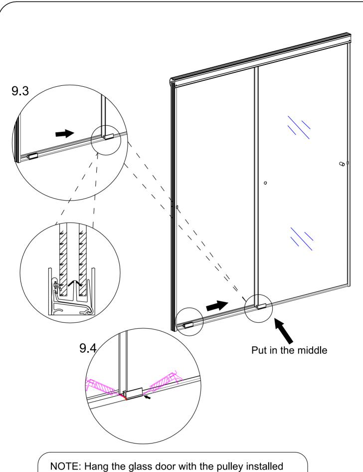
NOTE: Hang the glass door with the pulley installed into the top guide rail, then push the door to one side, slide the guide block on the guide rail to the middle of the guide rail, and respectively snap into the glass door. Put glass glue on both sides of the guide block.
