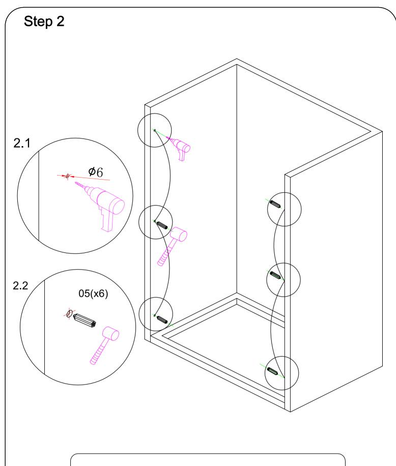
NOTE: Use the drill bit of Ø6 to drill the holes in turn against the marked holes, and then drive the expansion sleeve into each hole (#5).
