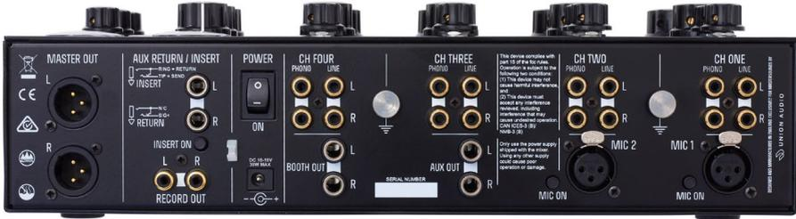
**MASTER OUT** – Output level is +14dBu when the MASTER level control is fully clockwise and the VU meters read -4VU. The XLR output is designed to operate with balanced equipment such as powered monitor speakers and amplifiers.
