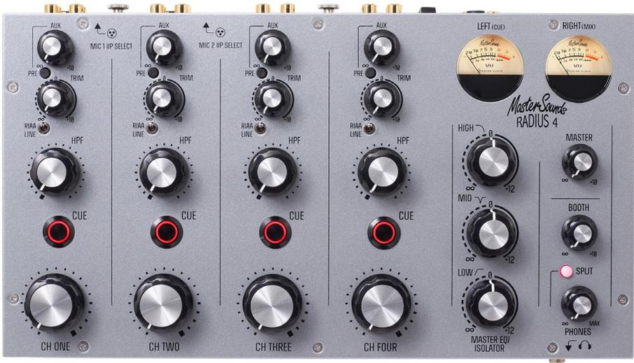
**AUX** – The AUX send level pot adjusts the amount of channel signal level sent to the Aux Mix Buss, (and on to an external FX unit). Fully clockwise the signal level is boosted by +10dBu, allowing for precise adjustment of FX signals.
