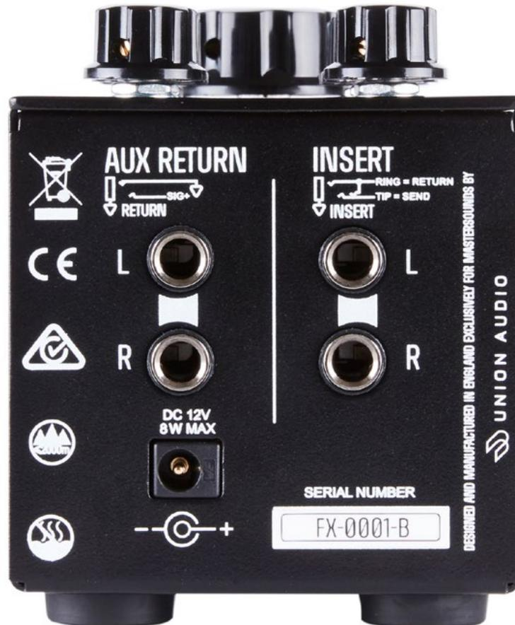
Each MasterSounds FX is supplied with four quality TRS jack leads. These are for connecting to your MasterSounds DJ mixer, and back into the FX.
