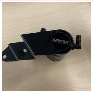
2. Using a 2.5mm hex key, remove the 3 screws from the top of the catch-can assembly. Align the bracket so that it is approximately at the 8 o'clock position relative to the etch Corsa logo atop the catch can and secure using the 3 screws and 2.5mm hex. Do not fully tighten the bolts at this time.
