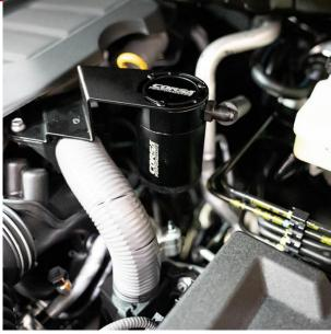
10. Adjust the rotation of the catch can assembly per the hose routing and fully tighten the 3 screws securing the catch can to the mounting bracket using a 2.5mm hex key.
