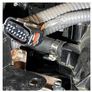
5. Slide the supplied #6 SAE hose clamp over the smaller 3" long hose. Next, slide the 3" long hose over the PCV fitting on the vehicle intake manifold, ensuring the hose is fully seated on the fitting. Position and secure the SAE #6 hose clamp over the hose and fitting using a ¼ socket.
