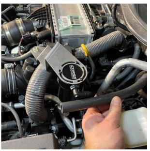
**6.** Route the open end of the 24" long x ½" hose along the firewall and to the B outlet fitting of the catch can assembly. Tiim away any excess length from the hose and insert it onto the fitting until the hose is fully seated.
