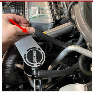
**9.** Route the open end of the 24" long x ½" hose along the firewall to the A inlet fitting of the catch can assembly. Trim away any excess length from the hose and insert it into the A inlet fitting until the hose is fully seated.
