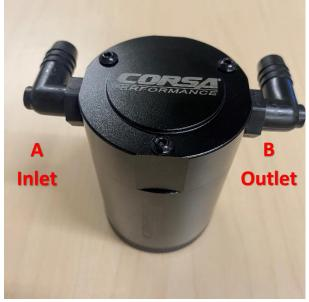
Install both 90 degree barb to 3/8" NPT fittings to the catch can using an 11/16" wrench. The barbed end of the fitting should be facing away from the vertical Corsa logo on the catch can body. IMPORTANT: Corsa highly recommends using thread sealant of PTFE tape on threaded fittings to prevent any leaks.
