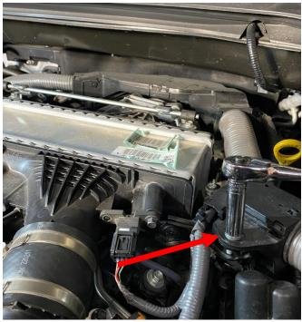
Using a ratchet and 10mm socket, remove the single bolt securing the main wiring harness just off to the driver side of the engine. Place the bolt in a safe location as if will be used during the installation of the catch can system.
