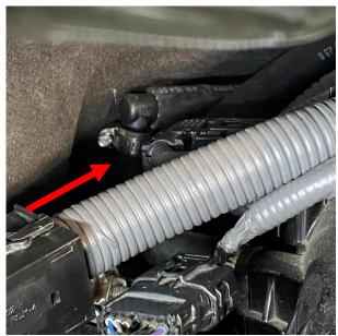
8. Slide the supplied SAE #6 hose clamp over the rubber PCV line located at the rear of the engine. Insert the 10mm barb portion into the vehicles PCV hose and secure using the SAE #6 clamp and 1/4" socket.
