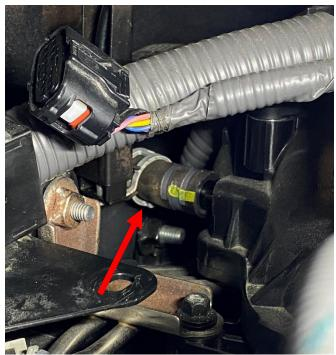
3. Locate where the PCV hose connects to the intake manifold at the rear of the engine. Loosen the constant tension clamp by squeezing the two tabs together and slide it down the hose. Carefully remove the rubber PCV hose from the fitting and then remove the constant tension clamp.
