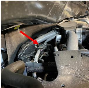
11. At this time, adjust the hose routing as necessary. If the wiring harness from step 2 of the removal portion of these instructions was disconnected, reconnect the wiring harness and secure it to the bracket.
