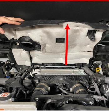
1. Remove the engine cover by pulling up from the front of the cover, then pulling out towards the front of the vehicle.
