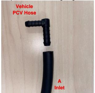
7. Locate the supplied 12mm to 10mm 90 degree barbed fitting, one of the two 24" long x ½" hoses and the stock constant tension clamp removed from step 3 of the removal portion of these instructions. Slide the constant tension clamp over one end of the ½" hose approximately 2" down. Insert the 12mm barb into the ½" hose until it is fully seated and secure with the clamp.
