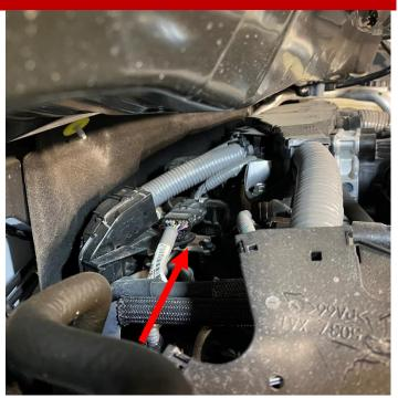
2. Looking at the rear of the engine, from the passenger side, locate the above pictured wiring harness connector. Remove the connector from the bracket, by squeezing the two tabs using a flat head screwdriver from underneath the bracket.
