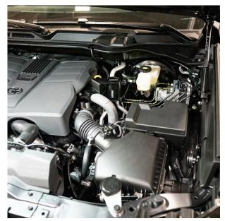
**12.** Reinstall the engine cover by first aligning and inserting the rear pivot points, then lower the front of the cover until the tabs click into place.
