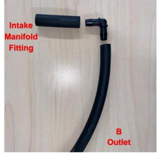
**4.** Locate the supplied ½" 90 degree barbed fitting, one of the two 24" long x ½" hoses and the smaller 3" long x ½" hose. Connect the two hoses using the fitting, ensuring the hoses are fully seated.
