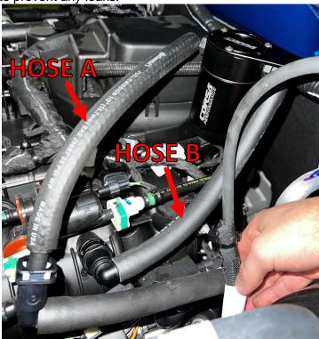
3. Install male barbed fitting to Hose A. Install female quick disconnect fitting to Hose B. Attach hose A to the "A" end of the catch can and route the hose to connect it to the stock PCV fitting. Connect Hose B to the "B" side of the catch can and route the line to connect it to fitting on the intake manifold. Make sure fittings are fully secured and the hose is pushed all the way over the ends of the fittings.
