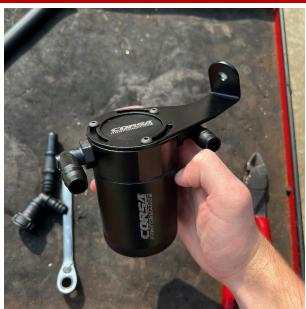
Install barbed fittings and bracket to the catch can using an 11/16" wrench and 2.5mm Hex wrench. IMPORTANT: Corsa recommends using thread sealant or PTFE tape on barbed fittings and bottom drain plug to prevent any leaks.
