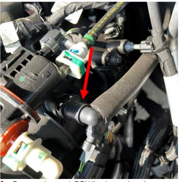
Remove the stock PCV line located on the drivers side of the engine by pressing on the grey tab.
