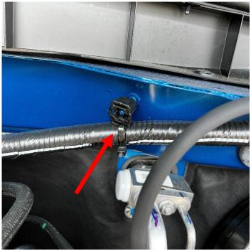
Located on the driver's side of the firewall, cut the zip tie securing the wiring harness to the plastic cap, then remove the plastic cap from the firewall stud.
