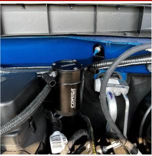
Use the provided nut and a 10mm socket ratchet or wrench to secure the catch can in place on the firewall stud.
