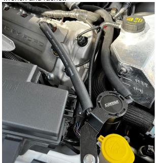
4. Connect the 2 quick disconnect fittings to one end of each hose. Attach hose A to the "A" end of the catch can and route to the BROWN fitting on the engine. Connect Hose B to the "B" side of the catch can and route it to the BLACK fitting on the engine. Reinstall engine cover.
