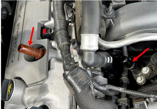
2. Remove stock PCV line which is located on the passenger side of the engine.
