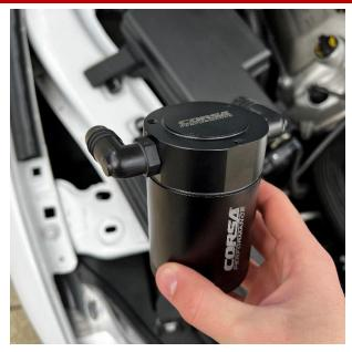
Install barbed fittings to the catch can using an 11/16" wrench. IMPORTANT: Corsa highly recommends using thread sealant or PTFE tape on barbed fittings and bottom drain plug to prevent any leaks.
