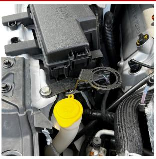
2. Use the supplied nut, bolt, and spacer to attach the bracket to the passenger side of the body above the windshield washer fluid cap. Place the spacer between the body panel and the bracket before tightening the nut/bolt using a 15mm wrench and rachet.
