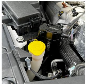
**3.** Install the catch can to the bracket using the provided hex screws and a 2.5mm Allen wrench.
