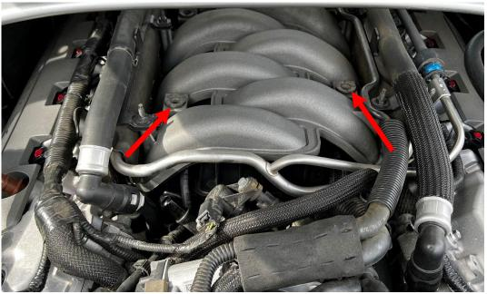
1. Remove the engine over by pulling it off of the press fit tabs.
