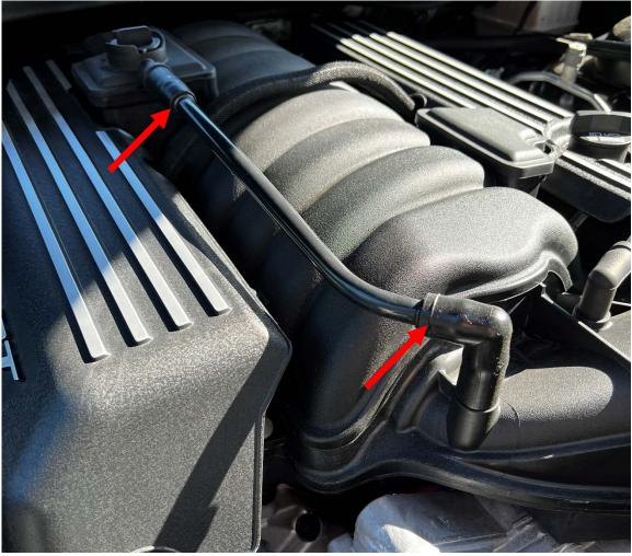
1. Locate the stock PCV line on top of the engine and remove it by pulling it off the rubber connections.
