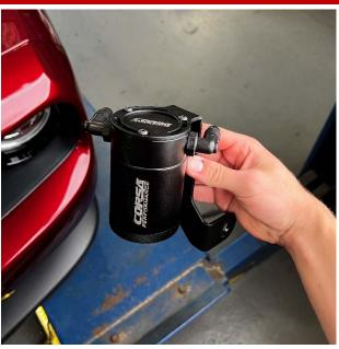
Install barbed fittings and bracket to the catch can using an 11/16" wrench and 2.5mm Hex wrench.
