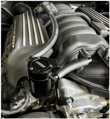
2. Use the provided nut and a 15mm socket wrench to secure the catch can bracket to the bolt extending off the front of the engine. Attach the 11" hose to the straight barbed fitting and route it to the A side of the catch can. Attach the 4" hose to the elbow barbed fitting and route it to the B side of the catch can.
