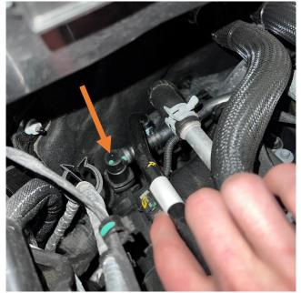
**3.** Locate and remove the opposite end of the PCV line attached to the crankcase on the back corner passenger side of the engine bay.
