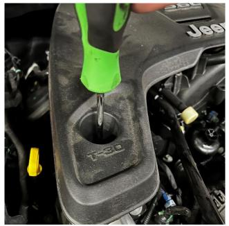
1. Remove the 2 screws that secure the engine cover using a T-30 Screwdriver. Pull the cover out towards the front of the car to remove it from the grommets holding it in place.
