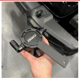
Use a 2.5mm Hex wrench to install the bracket in the orientation shown. Thread in barbed fittings by hand or by using an 11/16" wrench.
