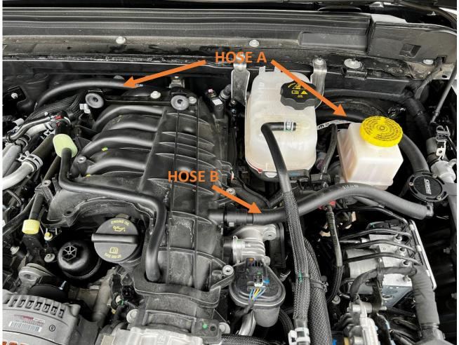
**5.** Make sure all fittings are secured in place and hose is pushed all the way over the barbed ends of the fittings. Reinstall engine cover.
