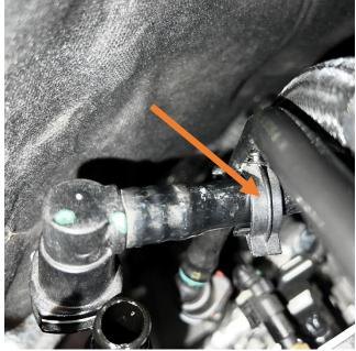
**4.** There are 4 clips attached along the PCV line. Detach PCV line from clips to remove the line from the vehicle.
