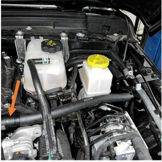
4. Connect the shorter hose to the intake manifold (see arrow) and attach the opposite end to port B of the catch can. You will hear a click when quick disconnect fittings are fully secured in place.
