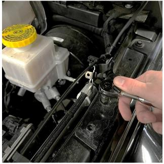
Using a 10mm socket, remove the bolt located next to the brake fluid reservoir on the driver's side. Install the catch can bracket using factory bolt to secure the catch can. Make sure the 90 degree fitting is installed in port B and straight fitting in port A of the can to properly route hose.
