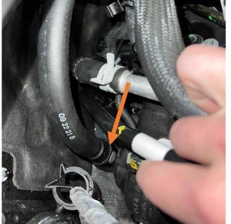
Attach quick disconnect fittings to 1 end of each hose. Attach Hose A to the crankcase side of the PCV system. Route the house back along the firewall and underneath the coolant reservoir and attach it to port A of the Catch can.
