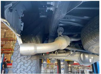
Using grommet pullers or a similar device, remove the axle pipe rear hanger located near the tailpipe outlet. NOTE: The use of soapy water solution will aid in the removal of the hanger grommets.
