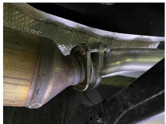
5. Locate the CORSA passenger side head-pipe and the flange, two M10 bolts, and lock washers from the hardware kit. Slide the flange over the pipe with the chamfer of the flange facing the pipe flare. Using a 14mm socket and ratchet, snug the flange and head-pipe to the factory catback flange.
