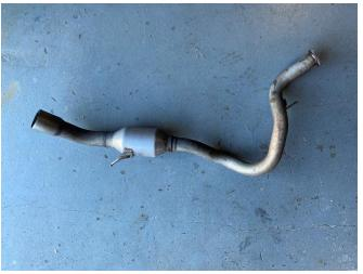
The axle pipe is now free. Maneuver the axle pipe rearward and over the vehicles axle.
