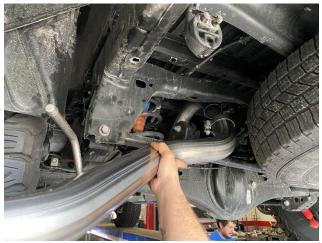
**10.** Locate, the Corsa tailpipe and one 3.0" clamp. Slide the clamp over the expanded end of the tailpipe with the clamp nut and bolt face the driver side of the vehicle and nut facing down. Slide the expanded end of the tailpipe over the axle pipe outlet.
