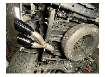
**12.** Locate the Corsa tip assembly and one 3.0" clamp. Slide the clamp over the expanded inlet end of the tip assembly so that the clamp nut and bolt is facing the rear tire with the bolt perpendicular to the ground. Using the 15mm socket and ratch, snug the clamp but do not fully tighten at this time.
