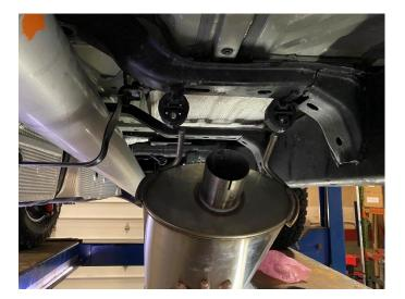
Locate the Corsa front muffler assembly. Slide the two hangers into the factory grommets.
