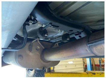
6. Using grommet pullers or a similar device, remove the two forward muffler hangers.
