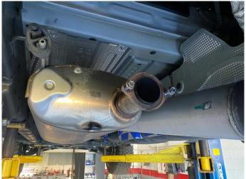
Using grommet pullers or a similar device, remove the rear muffler hanger. NOTE: The use of soapy water solution will aid in the removal of the hanger grommet.
