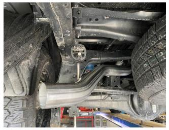
Insert the tailpipe hanger into the factory hanger grommet. Using a 15mm socket and ratchet, snug the clamp at the axle pipe to tailpipe connection. Do not fully tighten at this time.
