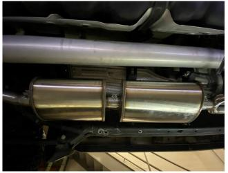
4. Install the expanded inlet end of the rear muffler onto the outlet of the front muffler. Snug the clamp using a 15mm socket and ratchet but do not fully tighten at this time.
