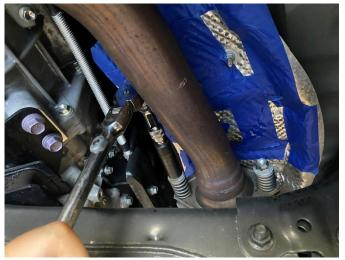
Moving to the front of the vehicle and using the ratchet and 14mm socket, remove the 4 bolts and springs located at the cat-back flanges on both he driver and passenger sides. NOTE: The use of penetrating lubricant spray on the rear of the threads may aid in removal.
