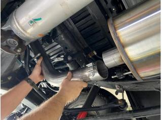
**9.** Locate the CORSA axle pipe and one 3.0" clamp. Insert the axle pipe hanger into the factory hanger grommet. Next, slide the 3" clamp over the expanded inlet end of the axle pipe inlet. Slide the axle pipe over the rear muffler outlet. Position the clamp so that the clamp nut and bolt are perpendicular to the ground and snug using a 15mm socket and ratchet.
