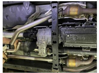
6. Locate the Corsa driver side head-pipe and two M10 bolts and lock-washers. Slide the floating flange to the flare on the head-pipe inlet and bolt it to the factory cat-back flange using the supplied M10 bolts, lock-washers and 14mm socket and ratchet.
