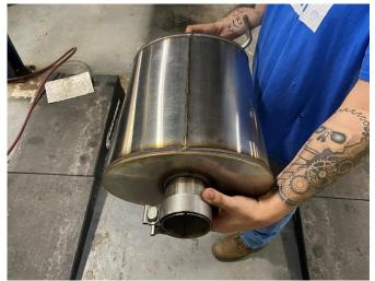
2. Locate the Corsa rear muffler assembly along with a 3" clamp. Slide the clamp over the expanded inlet side of the muffler with the nut and bolt perpendicular to the ground.
