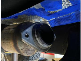
**9.** Inspect both the driver and passenger side exhaust gaskets left on the stock cat-back flanges for any cracking or damage and replace if necessary.
