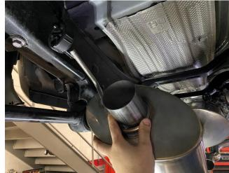
**3.** Slide the rear hanger into the factory rear muffler grommet.
