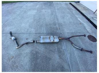
8. The rest of the factory exhaust system will come out in one piece. Slide the entire exhaust system down and rearwards to remove it from the vehicle.
