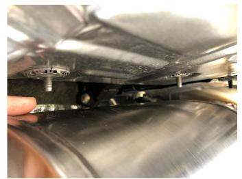
**25.** (FULL MUFFLER ONLY) Adjust the muffler position as needed until there is approximately a fingertip clearance between the heat shielding mounting studs and the top of the mufflers on both the driver and passenger side.
