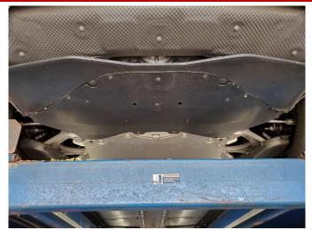
5. The forward most rear under tray is secured by one push clip and ten 7mm bolts. Remove the push clip first using a removal tool or flat head screwdriver. Next, remove the bolts using a 7mm socket and ¼" ratchet to free the forward under tray from the vehicle. Set aside the forward under tray and fasteners in a protected location.
