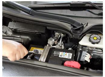
**3.** Disconnect the negative battery terminal using a 10mm socket and 1/4" ratchet.
