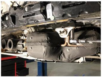
**21.** Support the factory exhaust with a jack stand. Remove the four bolts that secure both of the rear exhaust grommets to the chassis using a 13mm socket and 3/8" ratchet. Set aside the fasteners in a protected location.
