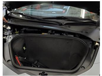
2. Unclip the front trunk battery cover panel and remove from the vehicle. Set the panel aside in a protected location.
