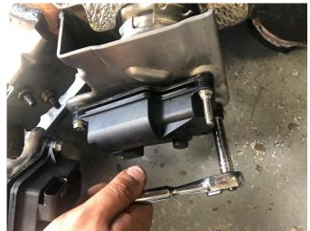
**31.** Repeat REMOVAL STEP 30 for the driver side factory NPP valve actuator using a 10mm socket and a ¼" ratchet for the one bolt and an 8mm socket and a ¼" ratchet for the two studs. Label and set aside the NPP valve actuator in a protected location. Both NPP valve actuators will be reused during the installation of the CORSA exhaust system.
