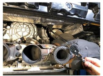
**23.** Remove the three M8 nuts that secure the passenger side cat back mounting flange to the factory catalyst using a 13mm socket, a 3/8" ratchet, and a 24" long extension. Set aside the fasteners in a protected location.
