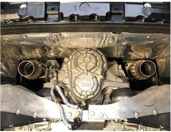
Pivot and rotate the CORSA driver side head pipe assembly at the flange connection until the head pipe position mirrors the passenger side on both height and rotation as shown.
