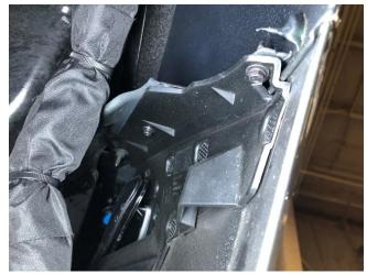
The sides of the rear bumper cover are secured to the quarter panel by a 10mm nut and two 7mm bolts on each side. Starting on the driver side, remove the nut first using a 10mm socket and 3/8" ratchet, followed by the two bolts using a 7mm socket and ¼" ratchet.
