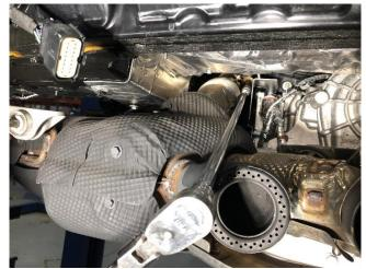
22. Remove the two M10 nuts that secure the driver side cat back mounting flange to the factory catalyst using a 15mm socket, a 3/8" ratchet, and a 24" long extension. Set aside the fasteners in a protected location.
