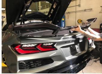
14. (FOR Z07 PACKAGE ONLY) (Continued) to free the rear wing from the vehicle. CAREFULLY set aside the Carbon Fiber rear wing and fasteners in a protected location.
