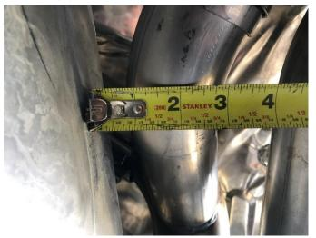
14. (FULL MUFFLER ONLY) Adjust the rotation and overlap of the center crossover assembly onto both head pipes until the outlets are even vertically, and each of the center crossover pipe to muffler outlet connections have approximately <sup>3</sup>/<sub>4</sub>" clearance from the front side of the pipe to the chassis as shown.
