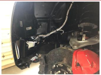
Repeat REMOVAL STEP 9 for the passenger side of the vehicle. Set aside both inner fender liners and fasteners in a protected location. REMOVAL STEPS 9-10 will allow access to the factory quarter panel to rear bumper cover connections on each side of the vehicle.
