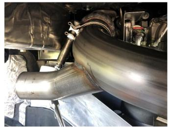
**15.** (FULL MUFFLER ONLY) Tighten both exhaust clamps at the driver and passenger side center crossover inlet connections using a 15mm socket and 3/8" ratchet to secure the center crossover assembly.
