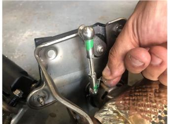
Remove the two locking pins from both NPP valve actuator linkages on the factory valve side (not valve actuator side) of the linkage as shown....
