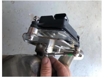
Locate the two locking pins set aside in REMOVAL STEPS 28/29. Connect both NPP valve actuator linkages to the CORSA NPP valve assemblies. Secure the connections with the locking pins.
