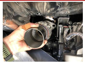
Locate the CORSA driver side head pipe assembly, and the two M10 nuts set aside in REMOVAL STEP 22. Insert the driver side CORSA head pipe assembly onto the studs from the catalyst as shown, then hand tighten the M10 nuts to hold the head pipe in place, leaving the nuts loose enough that the head pipe can still pivot and rotate.
