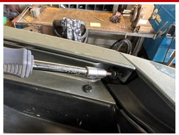
Remove the last two T15 TORX screws that are facing rearward and tucked into the corner of the fender on each side. This will allow the bumper cover to move independently from the vehicle. Set aside the fasteners in a protected location.
