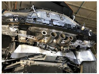
**33.** (MUFFLER DELETE ONLY) The CORSA muffler delete exhaust system should now be installed and positioned as shown.
