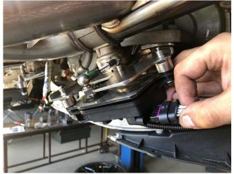
**<sup>35.</sup>** Connect the opposite end of the wiring extensions to the NPP valve actuators on both sides of the vehicle. Push in the grey locking tabs on the wiring connectors to secure the connections.
