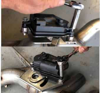
Locate the CORSA valved center crossover (or muffler delete) assembly, the two NPP valve actuators set aside in REMOVAL STEPS 30/31, and the six supplied M6 bolts. Identify driver and passenger side, then secure both factory NPP valve actuators to the CORSA NPP valve assemblies using a 10mm socket and a ¼" ratchet. Torque to 89 IN-LBS.
