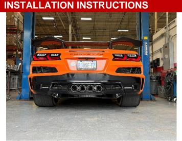
**37.** At this time, adjust the exhaust system position until all exhaust pipe outlets are centered within the collectors on the factory center exit tips, which are mounted to the rear valence.
