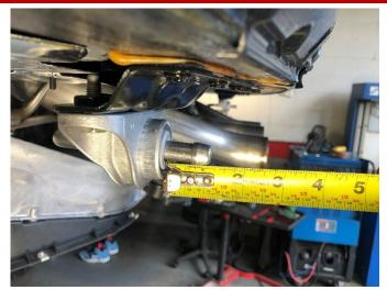
**31.** (MUFFLER DELETE ONLY) At this time, adjust the muffler delete and head pipe positions until there is approximately ½"- ¾" between the outer face of the rear grommets and the forward edge of the head on the rear hangers on both driver and passenger sides of the vehicle as shown. It is critical for proper fitment to get the system adjusted as square as possible on the vehicle.
