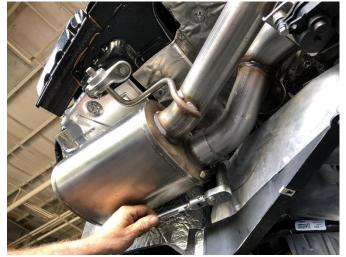
23. (FULL MUFFLER ONLY) Repeat INSTALL STEPS 16-22 for the driver side of the vehicle (CORSA driver muffler shown), then remove the supporting jack stand from under the exhaust.
