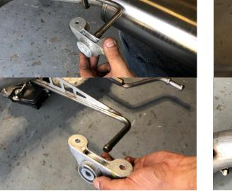
Locate both CORSA muffler assemblies (or the one-piece valved muffler delete assembly) and both rear grommets set aside in REMOVAL STEP 27. Install the rear exhaust grommets onto the rear hanger positions. Make sure the protruding rubber side of the grommet faces away from the piping (rearward) as shown.
