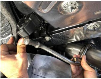
**28.** (MUFFLER DELETE ONLY) Insert both the driver and passenger side muffler delete front hangers into the front exhaust grommets as shown.
