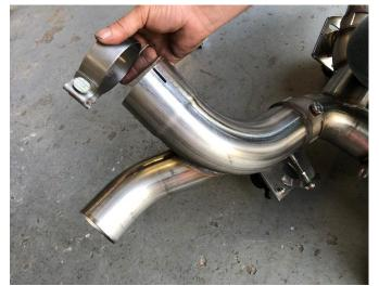
(FULL MUFFLER ONLY) Locate the two supplied 3" clamps. Position both clamps on the center crossover pipe inlets, so the clamp bolts are on the outside of the expansion and facing downwards as shown.
