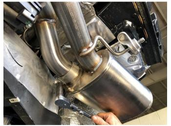
**22.** (FULL MUFFLER ONLY) Tighten the exhaust clamp at the passenger side muffler inlet connection using a 15mm socket and 3/8" ratchet to secure the passenger muffler assembly.
