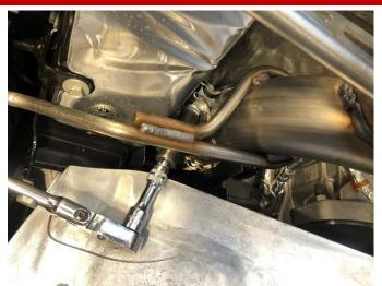
**32.** (MUFFLER DELETE ONLY) Tighten both exhaust clamps at the driver and passenger side muffler delete inlet connections using a 15mm socket and 3/8" ratchet to secure the muffler delete assembly.
