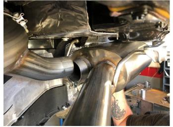
(FULL MUFFLER ONLY) Insert the inlet of the passenger muffler assembly on to the passenger side outlet of the center crossover assembly with approximately 1.375" of overlap.
