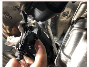
20. Disconnect the wiring connectors to both NPP valve actuators; these are located just in front of the pipes leading to the inner (center) exhaust position. Note that the grey locking tab on the wiring connectors must be slid outwards before disconnecting the wires from the actuators.
