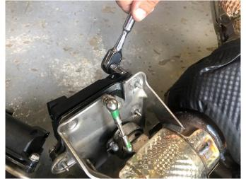
**30.** Remove the three bolts that secure the passenger side factory NPP valve actuator using a 10mm socket and a ¼" ratchet. Label the passenger side actuator accordingly to ensure that it is properly identified for the installation process, then set aside the NPP valve actuator in a protected location.
