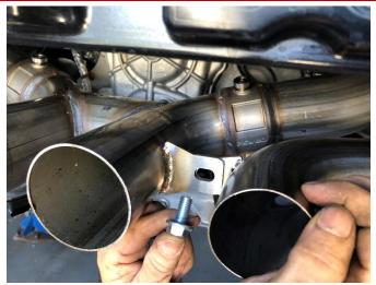
**20.** (FULL MUFFLER ONLY) Insert the M10 flange bolt through both slots in the tie brackets from the rearward side, and secure with the M10 flange nut. Snugly tighten with two 15mm wrenches, leaving it loose enough for later adjustment.
