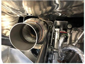
Next, secure the driver side cat back mounting flange to the factory catalyst using a 15mm socket, a 3/8" ratchet, and a 24" long extension. Torque to 32 FT-LBS.
