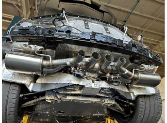
**26.** (FULL MUFFLER ONLY) The CORSA full muffler exhaust system should now be installed and positioned as shown.
