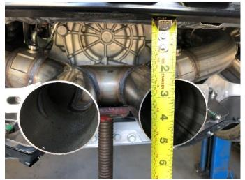
13. (FULL MUFFLER ONLY) Support the center of the CORSA center crossover assembly with a jack stand. Adjust the height of the jack stand until there is approximately a 2 ¼" gap between the top of the center crossover outlet and the chassis on both sides as shown.
