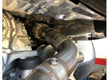
(FULL MUFFLER ONLY) Insert both inlet connections of the CORSA center crossover assembly on to the outlets of both head pipe assemblies, with approximately 1.75" of overlap at the pipe connection on both sides.
