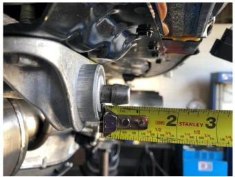
24. (FULL MUFFLER ONLY) At this time, adjust the muffler, center crossover, and head pipe positions until there is approximately ¼" between the outer face of the rear grommets and the forward edge of the head on the rear hangers on both driver and passenger sides of the vehicle as shown. It is critical for proper fitment to get the system adjusted as square as possible on the vehicle.
