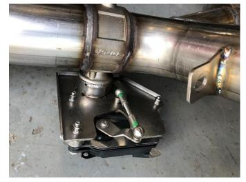
The NPP valve actuators should now be connected to the CORSA NPP valve assemblies as shown.
