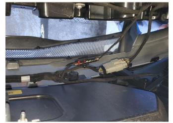
**19.** (Continued) followed by the two passenger side connectors to free the rear bumper cover from the vehicle. CAREFULLY set aside the factory rear bumper cover in a protected location.
