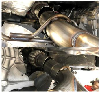
**29.** (MUFFLER DELETE ONLY) Insert both inlet connections of the CORSA muffler delete assembly on to the outlets of both head pipe assemblies, with approximately 1.75" of overlap at the pipe connection on both sides.
