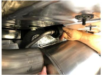
**17.** (FULL MUFFLER ONLY) Insert the passenger front muffler hanger into the front exhaust grommet as shown.
