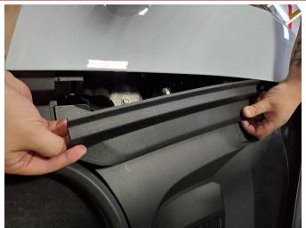
**1.** Beginning at the front of the vehicle, unclip the front trunk side panels and remove from the vehicle. Set the panels aside in a protected location.
