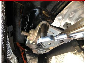
38. (IF NECESSARY) Additional side to side adjustment of the CORSA exhaust can be achieved by loosening the driver and passenger side rear grommet bolts using a 13mm socket and 3/8" ratchet, and then shifting the grommet position laterally until the desired position is achieved. Re-Torque fasteners to 17 FT-LBS.
