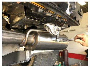
**21.** (FULL MUFFLER ONLY) Locate two of the factory rear grommet bolts set aside in REMOVAL STEP 21. Insert both bolts through the passenger rear exhaust grommet and secure the grommet to the chassis using a 13mm socket and 3/8" ratchet. Torque to 17 FT-LBS.
