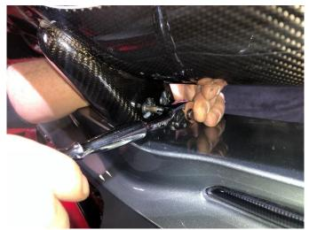
(FOR Z07 PACKAGE ONLY) Remove the four screws (2 per side) that secure the Carbon Fiber rear wing to the wing mounting blocks using a IPR30 TORX plus security bit and a ¼" ratchet...
