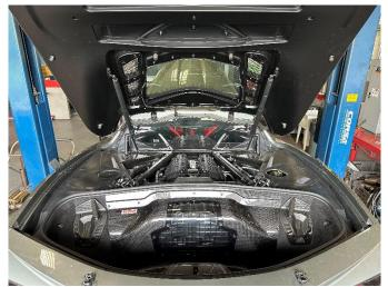
**16.** (ALL VERSIONS) Remove the sixteen T15 TORX screws that secure the top of the factory rear bumper cover to the chassis. Start with the fourteen screws that run along the top edge of the bumper.
