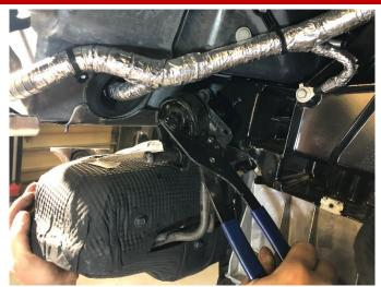
24. Remove both driver and passenger front exhaust grommets from the hanger on the chassis side of the connection using grommet pullers or similar device. The use of a soap and water solution will aid in the removal of the hangers from the factory grommets.
