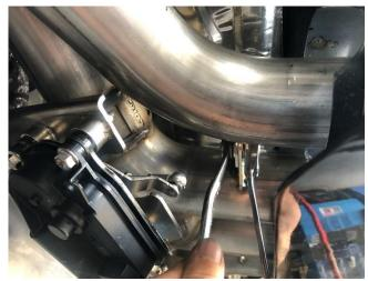
**39.** (IF NECESSARY) (FULL MUFFLER ONLY) Additional side to side muffler adjustment of the CORSA exhaust can be achieved by loosening both the tie bracket hardware, with two 15mm wrenches, and with the clamp at the muffler inlet, using a 15mm socket and 3/8" ratchet, then shifting the muffler position laterally until the desired position is achieved.
