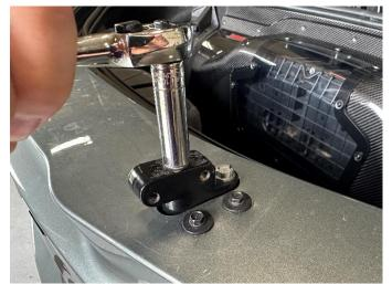
**15.** (FOR Z07 PACKAGE ONLY) The wing mounting blocks are secured by four bolts (2 per side). Remove the bolts to free the mounting blocks from the chassis using a 10mm socket and ¼" ratchet. This will allow the subsequent removal of the factory rear bumper cover from the vehicle. Set aside the fasteners in a protected location.
