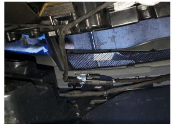
18. Get 2 helpers for REMOVAL STEPS 18 & 19. There are three wiring harness connectors that need to be disconnected to be able to remove the factory rear bumper cover from the vehicle. We recommend a person on each side of the vehicle CAREFULLY slide the rear bumper cover straight back and hold the bumper cover in the air while a third person disconnects the driver side connector....
