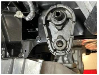
6. Locate both front grommets set aside in REMOVAL STEP 26. Reinstall both driver and passenger front exhaust grommets onto the hangers on the chassis side of the connections. Make sure the larger sides of the grommets face upward as shown.
