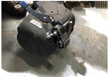
**26.** With the factory exhaust on the ground, remove the front grommets from the exhaust hangers using a grommet puller or similar device. Once again, the use of a soap and water solution will aid in the removal of the hangers from the factory grommets. Note the orientation of the grommets for the installation of the CORSA exhaust system. Set aside the grommets in a protected location.
