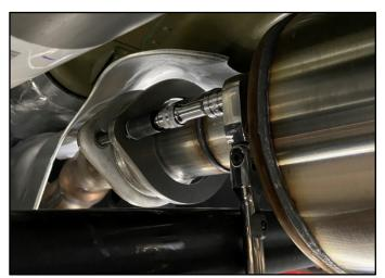
Locate the Head Flange Bolts from Removal Step 7. A second person may be needed to assist with this step.
