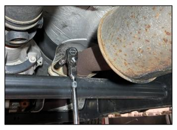
7. Use a 13mm Socket & Ratchet or Wrench to loosen the bolts from Stock Flange connection on the Front Section of the Stock exhaust. A second person may be needed to support the Front Section of the Stock exhaust.
