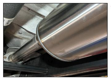
Locate 1 – 3in Clamp from the Hardware Kit and slide it over the Head Pipe. A second person may be needed to assist with this step.
