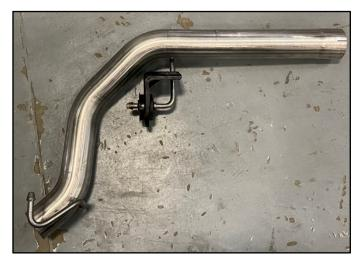
2. Locate the CORSA Front of Tire Tail Pipe. Install the Factory Grommet from Step 1 on to the Front Hanger, as shown. Make sure to orient the Factory Grommet as it was on the Factory exhaust.
