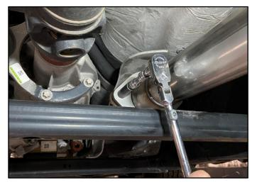
8. Locate the Head Flange Bolts from Removal Step 7. A second person may be needed to assist with this step.
