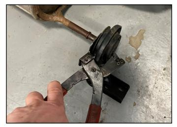
1. Using Grommet Pulling Pliers or similar, remove the Factory Grommets from the front of the Factory muffler. Note the orientation for the next step.
