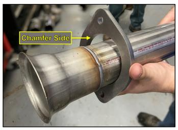
If installing a CORSA exhaust with a preassembled Head Pipe Flange on the muffler, skip to Step 10.
