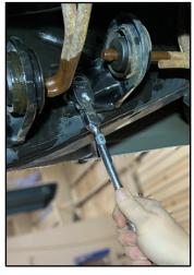
Use a 10mm Socket & Ratchet or Wrench to remove the 2 Bolts on each of the Factory Grommets. If the vehicle does not have the Flex Connector shown, the vehicle will have one Factory Grommet and may look different than shown.
