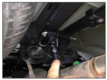
Using a 13mm Socket & Ratchet or Wrench, remove the 2 bolts attaching the factory Grommet to the Driver Rear Frame Rail.
