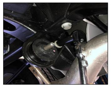
**11.** Using a 13mm Socket & Ratchet or Wrench, remove the 2 bolts attaching the factory Grommet to the Passenger Rear Frame Rail.
