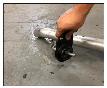
**13.** Remove the factory Grommet from factory Driver Tail Pipe Hanger and reattach it to the Frame using a 13mm Socket & Ratchet or Wrench.
