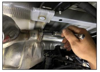
**8.** Loosen the factory flange on the Driver Tail Pipe using a 13mm Socket & Ratchet or Wrench.
