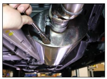
Using a 15mm socket & ratchet or wrench, SNUG the 3in Clamp.
