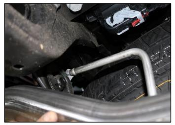
13. Insert the hanger on the CORSA Passenger Tail Pipe into the Grommet and insert the Tail Pipe outlet into the Factory Bezel opening.
