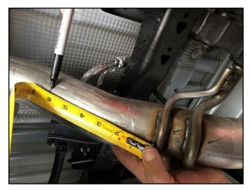
Mark a line 6" from the Hanger next to the muffler 2. closest to the rear of the vehicle.
