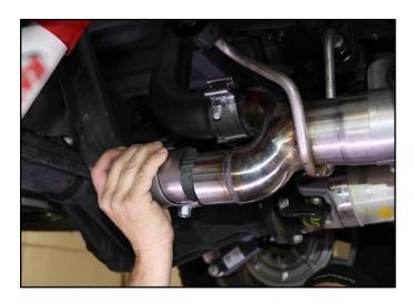
12. Lift the CORSA Passenger Axle Pipe over the vehicle's rear Axle and slide a supplied 2.5in Clamp over the Axle Pipe. Next, slide the Axle Pipe over the BOTTOM Wye Assembly outlet.
