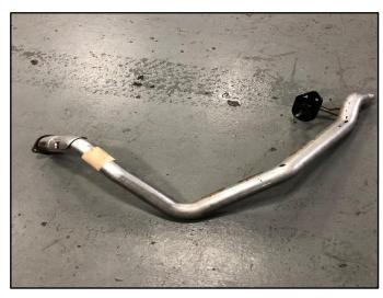
**10.** Remove the factory Driver Tail Pipe section.
