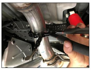
Place a Chain Style Cutter or similar around the exhaust pipe at the marked line location and cut the exhaust pipe.
