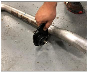
**14.** Remove the factory Grommet from factory Passenger Tail Pipe Hanger and reattach it to the Frame using a 13mm Socket & Ratchet or Wrench.
