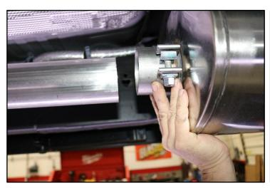
4. Slide a supplied 3.0in Clamp over the CORSA Head 5. Pipe (or 157in WB Extension). Then slide the Expanded end of the CORSA Muffler over the outlet of the Head Pipe (or 157in WB Extension).
