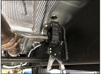
Remove the Grommets from the factory Head Pipe hangers at in the front of the muffler/behind the flex pipe, using Grommet Pulling Pliers or similar.
