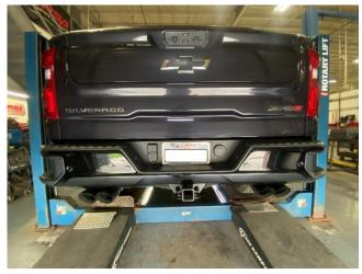
**18.** Verify the Tips are straight across and even. There should be approximately the same ½in gap all the around the Tips and Bezel openings. To adjust, you may need to loosen the Tail Pipe Clamps from Steps 14 and 15.
