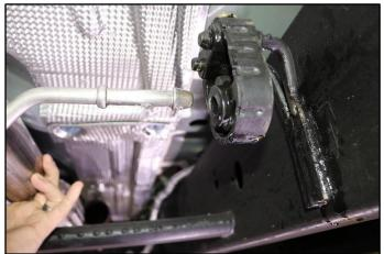
2. Insert the CORSA Head Pipe Hanger into the factory Head Pipe hanger grommet.
