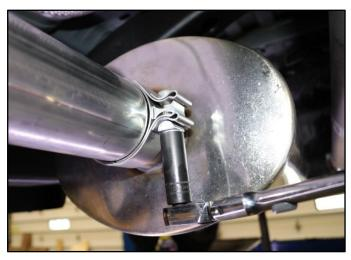
Using a 15mm socket & ratchet or wrench, SNUG 7. the 3in Clamp.
