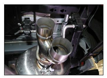
8. Insert the hangers on the Wye Assembly into the Grommets and then rotate and slide the expanded end of the Wye Assembly over the Muffler outlet.
