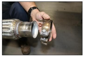
Locate the front section of the factory exhaust, and remove the Spherical Clamp by using a small flat screwdriver or similar and release the locking tab. Next, insert the Spherical Clamp onto the Head Pipe flare. Orient the Locking Tab facing the Flex Section.
