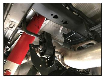
**5.** Remove the Grommet from the Driver Tail pipe Hanger behind the Muffler, using Grommet Pulling Pliers or similar.
