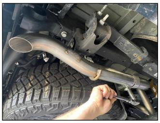
**14.** Slide a supplied 2.5in Clamp over the Passenger Tail Pipe. Next, rotate the Tail Pipe into position and slide the Expanded end of the Tail Pipe over the Axle Pipe.
