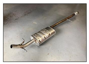
Remove the front section of the factory exhaust system and set it in a safe place. You will remove the Spherical Clamp in Install Step 1.
