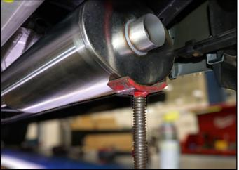
Support the rear of the CORSA Muffler with a Jack Stand or similar.
