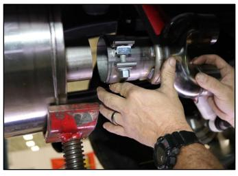
Slide a supplied 3in Clamp over the CORSA Wye Assembly, as shown.
