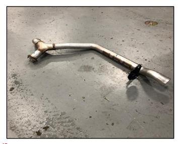
**12.** Remove the factory Passenger Tail Pipe and Wye section.
