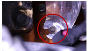
**13.** Remove the 8mm bolt on the starter's heat shield using an 8mm socket and ratchet. Save for **Install Step 5.**
