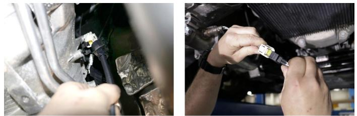
**21.** Locate the supplied zip ties and supplied driver rear O2 extension cable. Plug the O2 extension into the driver O2 harness and the other end into the O2 sensor. Tuck away any slack from any hot or moving parts.
