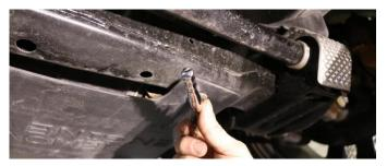
**13.** Reinstall plastic bottom engine cover using a 10mm socket and ratchet.
