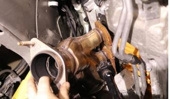
19. Remove the upper and lower driver side factory manifold bolts using a 10mm socket or wrench. Remove driver factory manifold from vehicle. PRO TIP: Remove middle two upper bolts first for easier access. It may be easier to access some of the manifold bolts from engine bay instead of underneath the vehicle.
