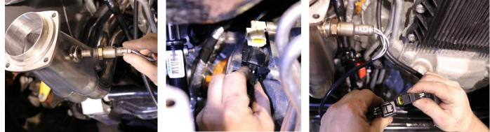
Insert the driver side front O2 sensor and tighten using an O2 socket or 22mm wrench. Install the supplied O2 extension cable into the front O2 wiring connector. Connect the O2 wiring harness and O2 extension.
