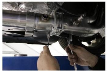
**17.** Install supplied hardware kit bolts and nuts and torque 15 ft-lbs using a torque wrench.
