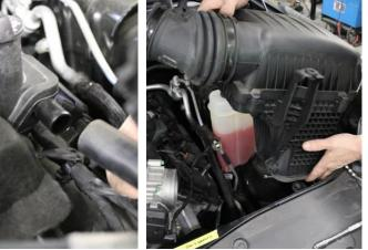
Disconnect the air intake vacuum tube and remove the factory air intake from the vehicle.
