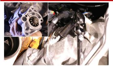
Unbolt and remove the starter using a 15mm socket and ratchet. Save bolts for Install Step 5.
