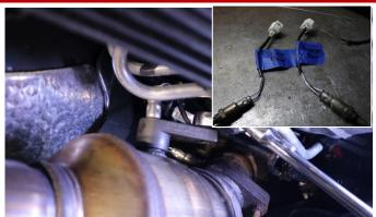
Remove the rear O2 sensors and label their positions using a 22mm wrench or O2 sensor socket and 3/8" ratchet. Save them for Install Step 22. PRO TIP: Label on the connector or the sensor body itself. EXAMPLE: DR for Driver Rear or PF for Passenger Front.
