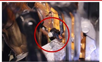
**18.** Remove the knock sensor from the driver side of engine block using a 13mm socket and ratchet.
