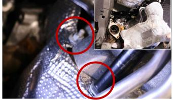
**14.** Remove the remaining 2 bolts on the starter's heat shield using a 13mm socket. Save heat shield and 3 bolts for **Install Step 5.**
