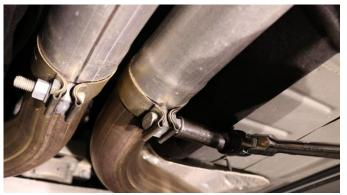
8. Using a 15mm socket, loosen the two nuts on the factory X-Pipe inlet.
