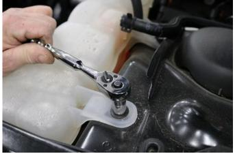
Unbolt the coolant reservoir using a 10mm socket and ratchet to allow easier access to the factory manifold bolts. Save bolt for Install Step 22. Lift and safely secure the vehicle.
