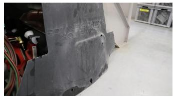
**1**. Remove the bottom plastic engine cover using a 10mm socket and ratchet.
