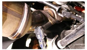
**9.** Using a 16mm socket and ratchet or wrench, remove the two nuts on the driver side catalytic converter flange. Repeat on passenger side.
