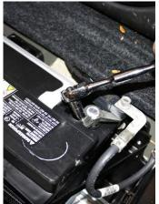
Lift the rear floor mat and the false floor up into the stowed position to allow access to the spare tire and battery compartment. Using a 10mm socket, disconnect the negative battery cable.
