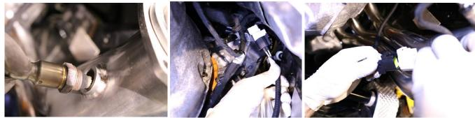
Insert the passenger front O2 sensor and tighten using an O2 socket or 22mm wrench. Install the supplied O2 extension cable into the front O2 wiring connector and connect the two together.
