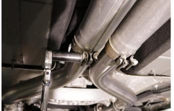
Tighten the inlet of the X-pipe clamps to factory specifications.
