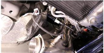
12. Tuck away the O2 sensor and extension wires using supplied zip ties and/or vehicle heat shielding. WARNING: DO NOT allow wires to contact the headers or other exhaust components.
