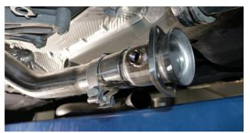
**16.** Add supplied clamp and flange adapter (20MU4171) to inlet of bent connection pipes (18LC4040 and 18LC4041). Rotate upwards until even with donut gasket.
