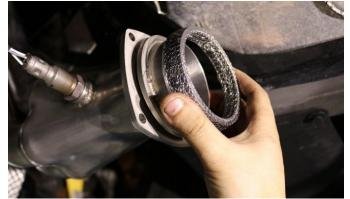
**14.** Install the supplied donut gaskets (99HK7000) to the outlet of the header collector.
