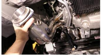
Lift the driver side CORSA header onto the 4 bottom bolts. Start the rest of the header bolts by hand and then torque to approximately 20FT LBS. Note: Gradually tighten all bolts because clearances are tight. Some bolts if left loose and not tightened gradually may contact header primaries if other bolts are fully tightened at the start.
