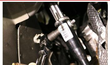
12. Mark the alignment of the steering shaft, located on the driver side of the vehicle. Remove the steering shaft bolt using a 10mm socket and ratchet. Save bolt for Install Step 10. Separate shaft and move out of the way. Do NOT turn or rotate the shaft while disconnected.
