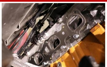
6. Prepare the remaining header bolts by applying a small amount of anti-seize to each of them. Insert 4 of the bolts through the lower holes in the provided OEM style stainless steel gasket as shown. WARNING: Hand start each bolt to prevent cross threading during installation.
