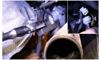
Unplug the front O2 sensor connectors. Remove the O2 sensors from the factory manifolds using a 22mm wrench or O2 sensor socket and 3/8" ratchet. Save for Install Step 4
