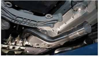
**15.** Slide outlet end of bent connection pipes (18LC4040 and 18LC4041) into the inlets of X-pipe.
