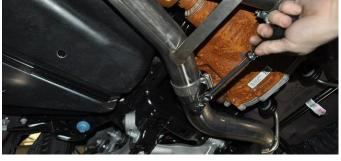
Once the system is secure, it is safe to remove the jack stand from beneath the X-Pipe
