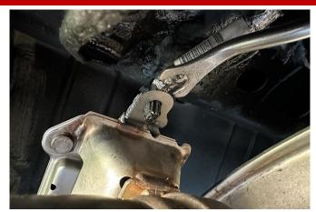
5. Use a push clip removal tool (or a flat head screwdriver) to remove the driver and passenger side Christmas tree fasteners (holding the valve actuator wiring harnesses to the anchor brackets) from the exhaust valves.
