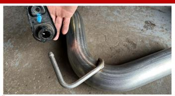
5. Locate the passenger side axle pipe assembly, and the hanger grommet assembly removed during **REMOVAL STEP 13** of the stock exhaust removal process. Install the hanger grommet assembly onto the front hanger of the muffler assembly in the same position as previously installed on the stock exhaust.
