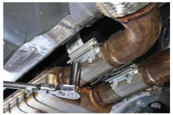
**8.** Use a 3/8" drive ratchet and 15mm deep socket to loosen both nuts on each of the two sleeve clamps as shown.
