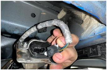
6. Unplug the wiring harness from the exhaust valve actuators located on the inner most driver and passenger tips. To release the plug, slide the white locking clip away from the actuator, press down on the clip and slide the plug away from the actuator.
