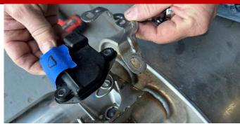
12. Use a 3/8" drive ratchet and a 10mm socket to remove the three nuts on each actuator. Remove the actuators from their valve assemblies. Place the actuators in a safe location to be used during INSTALL STEP 16. Install the hardware and anchor brackets back onto the studs or store in a safe location since they will NOT be re-used during installation.
