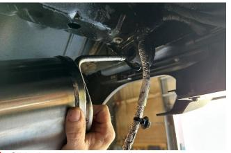
11. Slide the rear hanger into the rear hanger grommet located on the vehicle above and just inside of the passenger side tip cut out.
