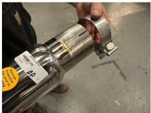
14. Locate one of the passenger non-valved tip assemblies and one 3" clamp. Install the clamp on the tip inlet pipe so that the bolt is vertical with the nut towards the ground and the bolt towards the outside of the vehicle.
