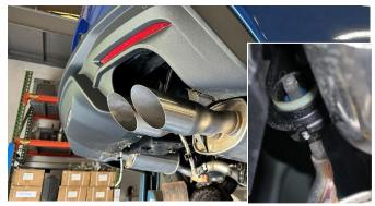
10. Slide the stock exhaust assembly rearward until the stock resonator and sleeve clamps are free from the exhaust manifold pipes. Lower the front of the exhaust then slide it forwards to remove the rear driver and passenger side hangers from their hanger grommets and remove the exhaust from the vehicle. NOTE: The use of a soap and water solution may aid in the removal of hangers from the grommets.
