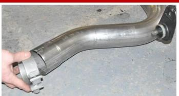
Locate one 3" clamp. Install the clamp on the passenger side muffler inlet pipe so that the bolt is vertical with the nut towards the ground and the bolt is towards the inside of the vehicle.
