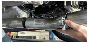
Slide the axle pipe inlet pipe over the passenger side X-pipe outlet. NOTE: The use of a soap and water solution may aid in the installation of hanger grommets.
