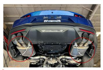
Both the driver and passenger side valve wiring harness connections should now be disconnected and hanging clear of the stock rear mufflers as shown.
