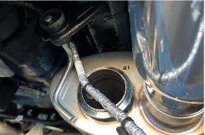
**18.** Reposition the driver and passenger valve actuator harnesses over their corresponding muffler hangers.
