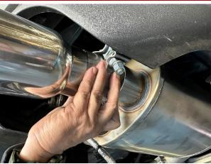
15. Slide the tip assembly over the muffler outlet pipe and tighten the clamp using the ratchet and 15mm deep socket until the tip assembly is snug on the muffler outlet pipe. Repeat for the driver side tip assembly.
