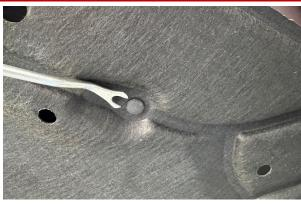
1. The rear under tray is secured by two push clips, one 10mm bolt, and seven 7mm bolts. Use a 1/4" drive ratchet and 10mm socket to remove the bolt securing the center of the rear under tray. Next, remove the two push clips using a removal tool or flat head screwdriver.
