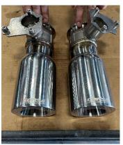
**16.** Confirm the spring wire form is correctly positioned on the passenger side stock valve actuator from **REMOVAL STEP 12**. Position and install passenger valve actuator onto the CORSA passenger valved tip assembly. Confirm that the spring wire form is located within the grooves of the valve assembly.
