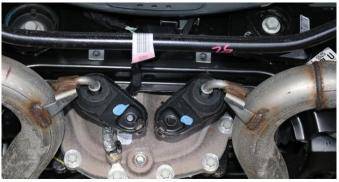
**9.** Use a 3/8" drive ratchet and 13mm socket to remove the bolt holding the driver side hanger grommet assembly. Push up slightly on the exhaust and slide the hanger grommet assembly rearward to free it from the rear suspension sub-frame. Rotate the hanger grommet assembly a minimum of 90° so it will not interfere with the rear suspension sub-frame. Repeat for passenger side. **Set aside the fasteners in a protected location to be reused in INSTALL STEP 8**.
