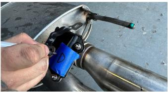
**11.** Place a piece of tape on each exhaust valve actuator and label them "D" for driver and "P" for passenger side.
