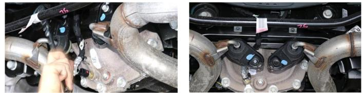
9. Use a 3/8" drive ratchet and 13mm socket to remove the bolt holding the driver side hanger grommet assembly. Push up slightly on the exhaust and slide the hanger grommet assembly rearward to free it from the rear suspension sub-frame. Rotate the hanger grommet assembly a minimum of 90° so it will not interfere with the rear suspension sub-frame. Repeat for passenger side. Set aside the fasteners in a protected location to be reused in INSTALL STEP 8.
