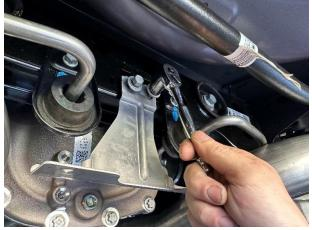
**13.** Locate the rear under tray mounting bracket and the two bolts set aside in **REMOVAL STEP 4** of the stock exhaust removal process. Install the rear under tray mounting bracket onto the rear suspension sub-frame and tighten it down with the two bolts using a 3/8" ratchet and 13mm socket.
