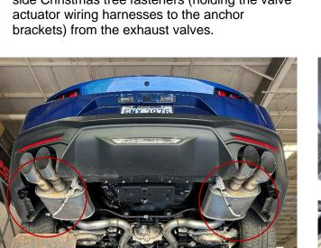
**1.** Both the driver and passenger side valve wiring harness connections should now be disconnected and hanging clear of the stock rear mufflers as shown.
