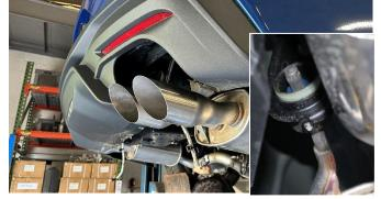
10. Slide the stock exhaust assembly rearward until the stock resonator and sleeve clamps are free from the exhaust manifold pipes. Lower the front of the exhaust then slide it forwards to remove the rear driver and passenger side hangers from their hanger grommets and remove the exhaust from the vehicle. NOTE: The use of a soap and water solution may aid in the removal of hangers from the grommets.
