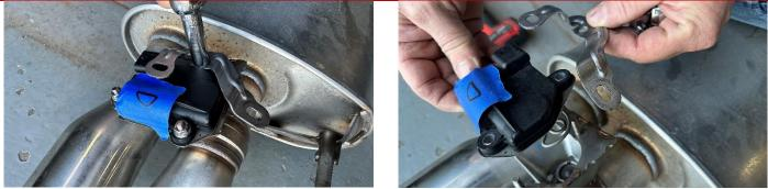
12. Use a 3/8" drive ratchet and a 10mm socket to remove the three nuts on each actuator. Remove the actuators from their valve assemblies. Place the actuators in a safe location to be used during INSTALL STEP 16. Install the hardware and anchor brackets back onto the studs or store in a safe location since they will NOT be re-used during installation.
