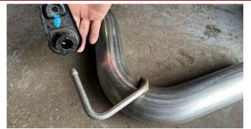
5. Locate the passenger side axle pipe assembly, and the hanger grommet assembly removed during REMOVAL STEP 13 of the stock exhaust removal process. Install the hanger grommet assembly onto the front hanger of the muffler assembly in the same position as previously installed on the stock exhaust.
