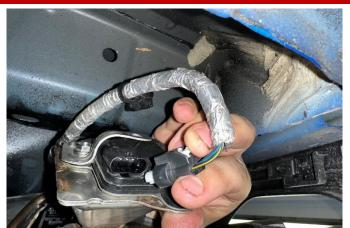
6. Unplug the wiring harness from the exhaust valve actuators located on the inner most driver and passenger tips. To release the plug, slide the white locking clip away from the actuator, press down on the clip and slide the plug away from the actuator.
