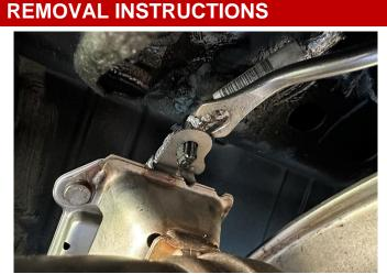
Use a push clip removal tool (or a flat head screwdriver) to remove the driver and passenger side Christmas tree fasteners (holding the valve actuator wiring harnesses to the anchor brackets) from the exhaust valves.
