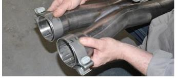
Install two 3" clamps on the driver and passenger inlets of the Double X-Pipe so that the bolts are vertical with the nut towards the ground and the bolts towards the outside of the vehicle.
