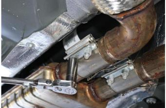
8. Use a 3/8" drive ratchet and 15mm deep socket to loosen both nuts on each of the two sleeve clamps as shown.
