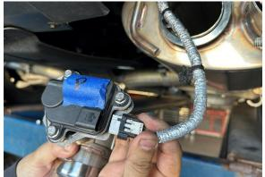
**19.** Connect the passenger side harness into the actuator mounted to the passenger valved tip assembly by pushing the plug until you hear a click, followed by the white locking clip. Once the actuator is secure, remove the "P" label from the actuator.
