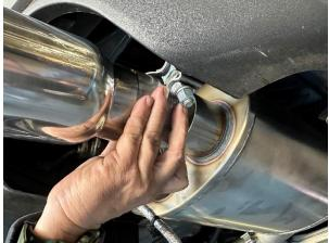
**15.** Slide the tip assembly over the muffler outlet pipe and tighten the clamp using the ratchet and 15mm deep socket until the tip assembly is snug on the muffler outlet pipe. Repeat for the driver side tip assembly.
