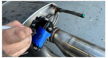
**11.** Place a piece of tape on each exhaust valve actuator and label them "D" for driver and "P" for passenger side.
