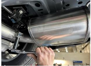
Slide the muffler inlet pipe over the passenger side axle pipe outlet. Tighten the clamp using the 3/8" ratchet and 15mm deep socket until the muffler assembly is snug on the axle pipe.
