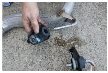
**13.** Remove the driver and passenger side hanger grommet assemblies from the axle pipe hangers using grommet pullers or a similar device. Save for **INSTALL STEP 5**.
