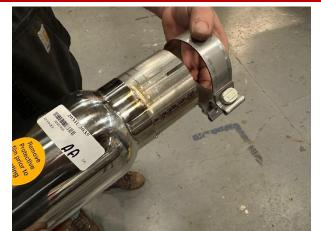
14. Locate one of the passenger non-valved tip assemblies and one 3" clamp. Install the clamp on the tip inlet pipe so that the bolt is vertical with the nut towards the ground and the bolt towards the outside of the vehicle.
