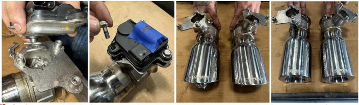
16. Confirm the spring wire form is correctly positioned on the passenger side stock valve actuator from REMOVAL STEP 12. Position and install passenger valve actuator onto the CORSA passenger valved tip assembly. Confirm that the spring wire form is located within the grooves of the valve assembly.
