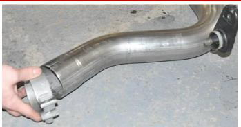
**6.** Locate one 3" clamp. Install the clamp on the passenger side muffler inlet pipe so that the bolt is vertical with the nut towards the ground and the bolt is towards the inside of the vehicle.
