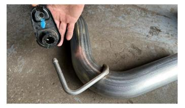
Locate the passenger side axle pipe assembly, and the hanger grommet assembly removed during REMOVAL STEP 14 of the stock exhaust removal process. Install the hanger grommet assembly onto the front hanger of the muffler assembly in the same position as previously installed on the stock exhaust.
