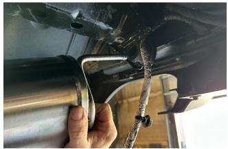
8. Slide the rear hanger into the rear hanger grommet located on the vehicle above and just inside of the passenger side tip cut out.
