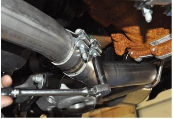
6. Tighten the clamp connecting the passenger axle pipe to the 3" adapter using the 3/8" ratchet and 15mm deep socket until the axle pipe assembly is snug on the adapter.
