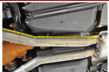
8. Measure 20" away from the flange on the stock resonator, following the outside profile of the exhaust pipe of the passenger side.
