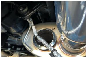
**15.** Reposition the driver and passenger valve actuator harnesses over their corresponding muffler hangers.
