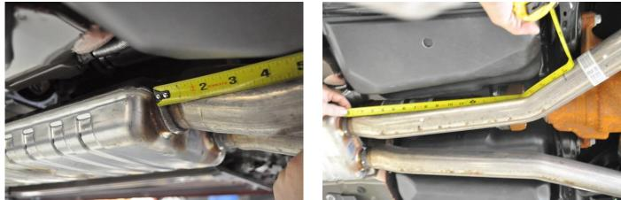
**7.** Starting on the driver side, measure 19 <sup>3</sup>/<sub>4</sub>" away from the flange on the stock resonator, following the outside profile of the exhaust pipe. The tape measure should follow the bend profile of the pipe.
