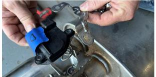
13. Use a 3/8" drive ratchet and a 10mm socket to remove the three nuts on each actuator. Remove the actuators from their valve assemblies. Place the actuators in a safe location to be used during INSTALL STEP 13. Install the hardware and anchor brackets back onto the studs or store in a safe location since they will NOT be re-used during installation.
