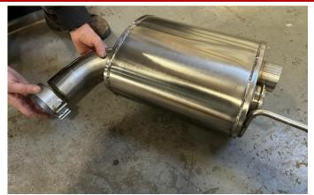
Locate the passenger side muffler assembly and one 3" clamp. Install the clamp on the muffler inlet pipe so that the bolt is vertical with the nut towards the ground and the bolt is towards the muffler case (facing the rear of the vehicle).
