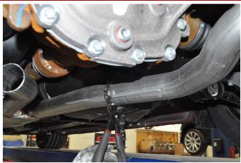
9. Using a chain cutter or similar device, cut both the driver and passenger side exhaust pipes at the marked locations. Place a jack stand or similar device under the stock tunnel section of the exhaust for support. Once the axle pipes are cut, there are no additional stock hangers supporting the tunnel section.
