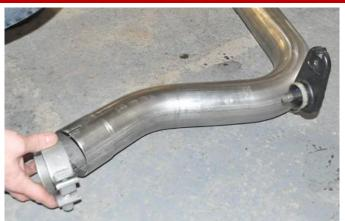
**3.** Locate one 3" clamp. Install the clamp on the passenger side axle pipe so that the bolt is vertical with the nut towards the ground and the bolt is towards the inside of the vehicle
