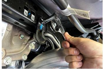
Locate a 13mm bolt set aside during REMOVAL STEP 10 of the stock exhaust removal process. Install the front passenger hanger grommet assembly onto the rear suspension sub-frame and tighten it down with the 13mm bolt, 3/8" ratchet and 13mm socket.
