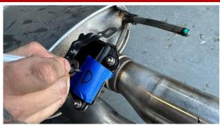
**12.** Place a piece of tape on each exhaust valve actuator and label them "D" for driver and "P" for passenger side.
