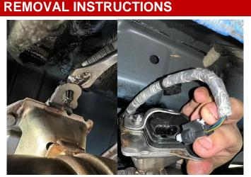
5. Use a push clip removal tool, or a flat head screwdriver to remove the driver and passenger side Christmas tree fasteners (holding the valve actuator wiring harnesses to the anchor brackets) from the exhaust valves. Next, unplug the wiring harness from the exhaust valve actuators located on the inner most driver and passenger tips. To release the plug, slide the white locking clip away from the actuator, press down on the clip and slide the plug away from the actuator.
