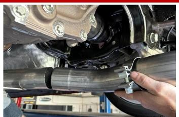
Slide the axle pipe inlet pipe over the passenger side adapter. NOTE: The use of a soap and water solution may aid in the installation of hanger grommets.
