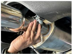
Slide the tip assembly over the muffler outlet pipe and tighten the clamp using the ratchet and 15mm deep socket until the tip assembly is snug on the muffler outlet pipe. Repeat for the driver side tip assembly.
