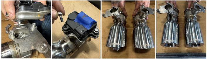
13. Confirm the spring wire form is correctly positioned on the passenger side stock valve actuator from REMOVAL STEP 13. Position and install passenger valve actuator onto the CORSA passenger valved tip assembly. Confirm that the spring wire form is located within the grooves of the valve assembly.
