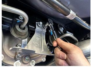
Locate the rear under tray mounting bracket and the two bolts set aside in REMOVAL STEP 4 of the stock exhaust removal process. Install the rear under tray mounting bracket onto the rear suspension sub-frame and tighten it down with the two bolts using a 3/8" ratchet and 13mm socket.
