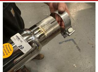
**11.** Locate one of the passenger non-valved tip assemblies and one 3" clamp. Install the clamp on the tip inlet pipe so that the bolt is vertical with the nut towards the ground and the bolt towards the outside of the vehicle.
