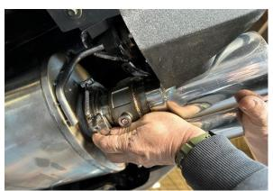
14. Line up the holes on the passenger actuator to the threaded spacers on the valve assembly.
