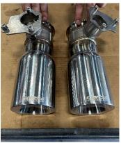
**13.** Confirm the spring wire form is correctly positioned on the passenger side stock valve actuator from **REMOVAL STEP 13**. Position and install passenger valve actuator onto the CORSA passenger valved tip assembly. Confirm that the spring wire form is located within the grooves of the valve assembly.
