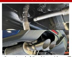
11. Lower the cut end of the driver side muffler assembly just enough to create clearance between the pipe and any suspension components. Slide the whole muffler assembly forward to remove the rear muffler hanger from the hanger grommet. The driver muffler assembly will now be free from the vehicle. NOTE: The use of a soap and water solution may aid in the removal of the hanger grommets. Repeat REMOVAL STEPS 10-11 for the passenger side.
