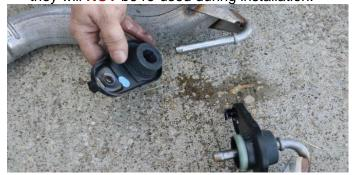
14. Remove the driver and passenger side hanger grommet assemblies from the axle pipe hangers using grommet pullers or a similar device. Set aside the hanger grommet assemblies to be reused in INSTALL STEP 2.
