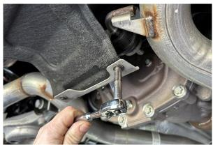
2. Use a 1/4" drive ratchet and 7mm socket to remove the two bolts securing the forward end of the rear under tray.
