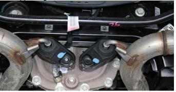
10. Use a 3/8" drive ratchet and 13mm socket to remove the bolt holding the driver side hanger grommet assembly. Push up slightly on the exhaust and slide the hanger grommet assembly rearward to free it from the rear suspension sub-frame. Rotate the hanger grommet assembly a minimum of 90° so it will not interfere with the rear suspension sub-frame. Set aside the fastener in a protected location to be reused in INSTALL STEP 5.
