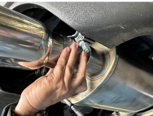
12. Slide the tip assembly over the muffler outlet pipe and tighten the clamp using the ratchet and 15mm deep socket until the tip assembly is snug on the muffler outlet pipe. Repeat for the driver side tip assembly.
