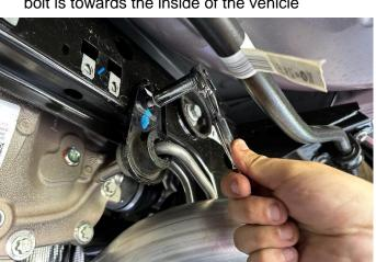
j. Locate a 13mm bolt set aside during REMOVAL STEP 10 of the stock exhaust removal process. Install the front passenger hanger grommet assembly onto the rear suspension sub-frame and tighten it down with the 13mm bolt, 3/8" ratchet and 13mm socket.
