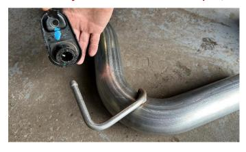
2. Locate the passenger side axle pipe assembly, and the hanger grommet assembly removed during REMOVAL STEP 14 of the stock exhaust removal process. Install the hanger grommet assembly onto the front hanger of the muffler assembly in the same position as previously installed on the stock exhaust.
