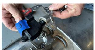
**13.** Use a 3/8" drive ratchet and a 10mm socket to remove the three nuts on each actuator. Remove the actuators from their valve assemblies. Place the actuators in a safe location to be used during **INSTALL STEP 13.** Install the hardware and anchor brackets back onto the studs or store in a safe location since they will **NOT** be re-used during installation.
