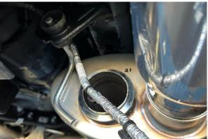
Reposition the driver and passenger valve actuator harnesses over their corresponding muffler hangers.
