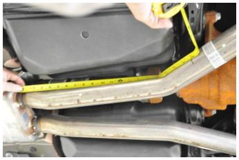
7. Starting on the driver side, measure 19 3/4" away from the flange on the stock resonator, following the outside profile of the exhaust pipe. The tape measure should follow the bend profile of the pipe.
