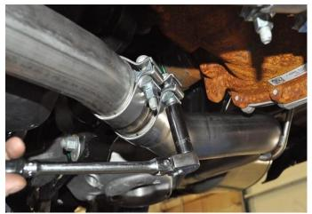
f. Tighten the clamp connecting the passenger axle pipe to the 3" adapter using the 3/8" ratchet and 15mm deep socket until the axle pipe assembly is snug on the adapter.
