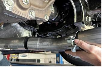
4. Slide the axle pipe inlet pipe over the passenger side adapter. NOTE: The use of a soap and water solution may aid in the installation of hanger grommets.
