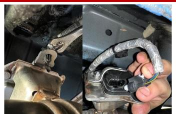
5. Use a push clip removal tool, or a flat head screwdriver to remove the driver and passenger side Christmas tree fasteners (holding the valve actuator wiring harnesses to the anchor brackets) from the exhaust valves. Next, unplug the wiring harness from the exhaust valve actuators located on the inner most driver and passenger tips. To release the plug, slide the white locking clip away from the actuator, press down on the clip and slide the plug away from the actuator.
