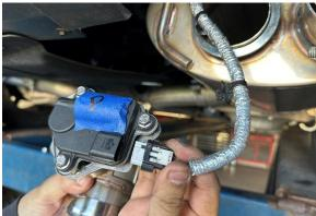
16. Connect the passenger side harness into the actuator mounted to the passenger valved tip assembly by pushing the plug until you hear a click, followed by the white locking clip. Once the actuator is secure, remove the "P" label from the actuator.
