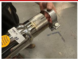
11. Locate one of the passenger non-valved tip assemblies and one 3" clamp. Install the clamp on the tip inlet pipe so that the bolt is vertical with the nut towards the ground and the bolt towards the outside of the vehicle.
