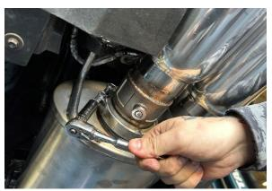
17. Mate the v-band flange on the driver valve tip assembly to the flange on the muffler. Align and position the v-band flange so both flanges are fitted within the grooves of the clamp. Reinstall the lock nut and snug the clamp using an 11mm deep socket and 3/8" drive ratchet. The clamp should be positioned with the lock nut towards the inside of the vehicle, the bolt on top and horizontal.
