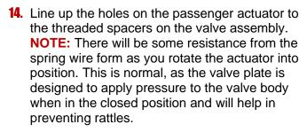
Use a 10mm socket and 3/8" drive ratchet to secure the valve actuator with the three provided M6 bolts with a blue Loctite patches. Repeat **INSTALL STEPS 13-14** for the driver side valved tip assembly.
