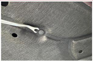
The rear under tray is secured by two push clips, one 10mm bolt, and seven 7mm bolts. Use a 1/4" drive ratchet and 10mm socket to remove the bolt securing the center of the rear under tray. Next, remove the two push clips using a removal tool or flat head screwdriver.
