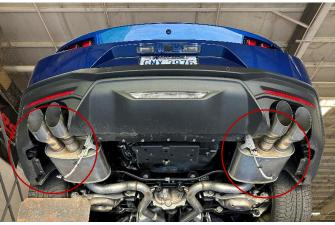
6. Both the driver and passenger side valve wiring harness connections should now be disconnected and hanging clear of the stock rear mufflers as shown.
