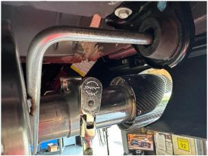
13. Locate the passenger rear tip assembly and one 3" clamp. Install the clamp on the tip inlet pipe so that the bolt is horizontal with the nut towards the inside of the vehicle and the bolt towards the top. Slide the tip assembly over the muffler outlet pipe and tighten the clamp using the ratchet and 15mm deep socket until the tip assembly is snug on the muffler outlet pipe. Repeat for the driver side tip assembly.
