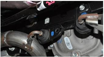
5. Once the bolt is removed, push up slightly on the exhaust and slide the hanger grommet assembly rearward to free it from the rear suspension subframe. Rotate the hanger grommet assembly a minimum of 90° so that it will not interfere with the rear suspension sub-frame. Repeat for the passenger side hanger grommet assembly. Set aside the fasteners in a protected location to be reused in INSTALL STEP 8.
