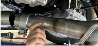
Slide the axle pipe inlet pipe over the passenger side X-pipe outlet. NOTE: The use of a soap and water solution may aid in the installation of hanger grommets.
