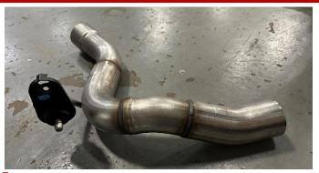
5. Locate the passenger side axle pipe assembly, and the hanger grommet assembly removed during REMOVAL STEP 7 of the stock exhaust removal process. Install the hanger grommet assembly onto the front hanger of the muffler assembly in the same position as previously installed on the stock exhaust.
