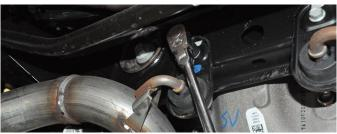
Use a 3/8" drive ratchet and 13mm socket, to remove the bolt holding down the driver side hanger grommet assembly.
