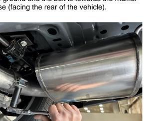
12. Slide the muffler inlet pipe over the passenger side axle pipe outlet. Tighten the clamp using the 3/8" ratchet and 15mm deep socket until the muffler assembly is snug on the axle pipe.
