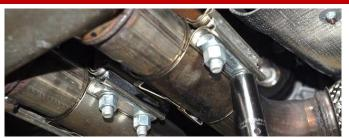
**3.** Use a 3/8" drive ratchet and 15mm deep socket, to loosen the two sleeve clamps at the cat-back connection point. Both nuts must be loosened in order for the clamp to fully disengage.
