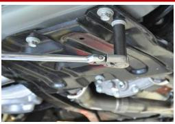
1. Loosen the furthest front bolt holding the driver side factory convertible brace using a 3/8" drive ratchet and 13mm deep socket. Loosen the bolt so there is about a ½" – ½" gap between the bolt head and the brace. Do not remove the bolt completely. Remove the factory driver side convertible brace by removing the remaining 7 bolts, working your way from front to rear; then slightly lowering the brace and sliding it rear wards.
