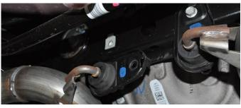
7. Once the bolt is removed, push up slightly on the exhaust and slide the hanger grommet assembly rearward to free it from the rear suspension subframe. Rotate the hanger grommet assembly a minimum of 90° so that it will not interfere with the rear suspension sub-frame.
