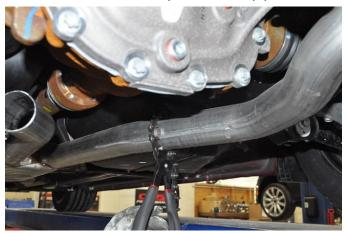
5. Using a chain cutter or similar device, cut both the driver and passenger side exhaust pipes at the marked locations. Place a jack stand or similar device under the stock tunnel section of the exhaust for support. Once the axle pipes are cut, there are no additional stock hangers supporting the tunnel section.
