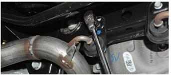
6. Using a 3/8" drive ratchet and 13mm socket, remove the bolt holding down the driver side hanger grommet assembly. Set aside the fastener in a protected location to be reused in INSTALL STEP 5.
