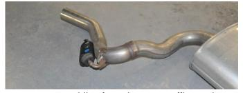
9. Remove both the driver and passenger side hanger grommet assemblies from the rear mufflers using grommet pullers or a similar device. Set aside the hanger grommet assemblies to be reused in INSTALL STEP 2.
