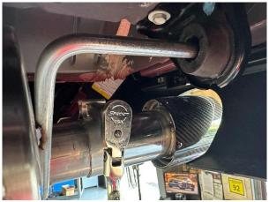
10. Locate the passenger rear tip assembly and one 3" clamp. Install the clamp on the tip inlet pipe so that the bolt is horizontal with the nut towards the inside of the vehicle and the bolt towards the top. Slide the tip assembly over the muffler outlet pipe and tighten the clamp using the ratchet and 15mm deep socket until the tip assembly is snug on the muffler outlet pipe. Repeat for the driver side tip assembly.
