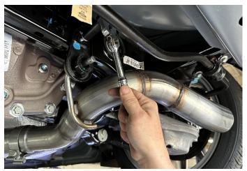
5. Locate a 13mm bolt set aside during REMOVAL STEP 6 of the stock exhaust removal process. Install the front passenger hanger grommet assembly onto the rear suspension sub-frame and tighten it down with the 13mm bolt, 3/8" ratchet and 13mm socket.
