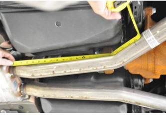
**3.** Starting on the driver side, measure 19 ¾" away from the flange on the stock resonator, following the outside profile of the exhaust pipe. The tape measure should follow the bend profile of the pipe.
