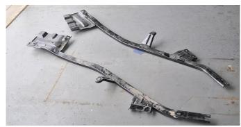
Repeat INSTALL STEP 1 on the passenger side of the vehicle. Set aside the fasteners and convertible bracing in a protected location to be reused in INSTALL STEP 12.
