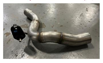
2. Locate the passenger side axle pipe assembly, and the hanger grommet assembly removed during REMOVAL STEP 9 of the stock exhaust removal process. Install the hanger grommet assembly onto the front hanger of the muffler assembly in the same position as previously installed on the stock exhaust.
