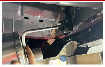
8. Slide the rear hanger into the rear hanger grommet located on the vehicle above and just inside of the passenger side tip cut out.
