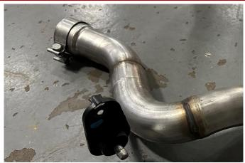
**3.** Locate one 3" clamp. Install the clamp on the passenger side axle pipe so that the bolt is vertical with the nut towards the ground and the bolt is towards the inside of the vehicle
