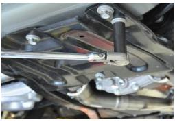
1. Loosen the furthest front bolt holding the driver side factory convertible brace using a 3/8" drive ratchet and 13mm deep socket. Loosen the bolt so there is about a  $\frac{1}{4}$ " –  $\frac{1}{2}$ " gap between the bolt head and the brace. Do not remove the bolt completely. Remove the factory driver side convertible brace by removing the remaining 7 bolts, working your way from front to rear; then slightly lowering the brace and sliding it rear wards.
