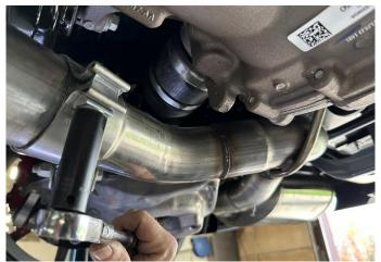
fi. Tighten the clamp connecting the passenger axle pipe to the 3" adapter using the 3/8" ratchet and 15mm deep socket until the axle pipe assembly is snug on the adapter.
