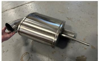
1. Locate the passenger side muffler assembly and one 3" clamp. Install the clamp on the muffler inlet pipe so that the bolt is vertical with the nut towards the ground and the bolt is towards the muffler case (facing the rear of the vehicle).
