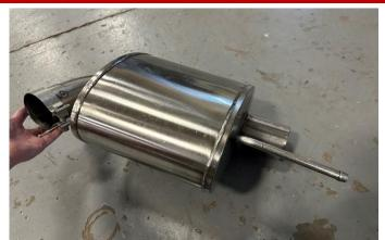
10. Locate the passenger side muffler assembly and one 3" clamp. Install the clamp on the muffler inlet pipe so that the bolt is vertical with the nut towards the ground and the bolt is towards the muffler case (facing the rear of the vehicle).
