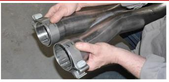
2. Install two 3" clamps on the driver and passenger inlets of the Double X-Pipe so that the bolts are vertical with the nut towards the ground and the bolts towards the outside of the vehicle.
