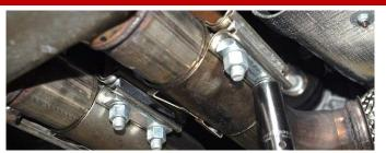
**5.** Use a 3/8" drive ratchet and 15mm deep socket, to loosen the two sleeve clamps at the cat-back connection point. Both nuts must be loosened in order for the clamp to fully disengage.
