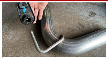
5. Locate the passenger side axle pipe assembly, and the hanger grommet assembly removed during REMOVAL STEP 9 of the stock exhaust removal process. Install the hanger grommet assembly onto the front hanger of the muffler assembly in the same position as previously installed on the stock exhaust.
