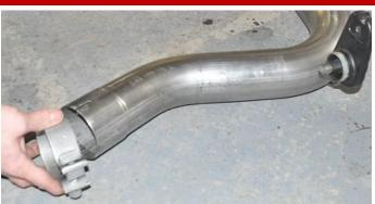
b. Locate one 3" clamp. Install the clamp on the passenger side muffler inlet pipe so that the bolt is vertical with the nut towards the ground and the bolt is towards the inside of the vehicle.
