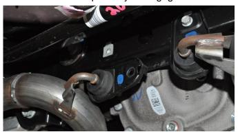
7. Once the bolt is removed, push up slightly on the exhaust and slide the hanger grommet assembly rearward to free it from the rear suspension subframe. Rotate the hanger grommet assembly a minimum of 90° so that it will not interfere with the rear suspension sub-frame. Repeat for the passenger side hanger grommet assembly. Set aside the fasteners in a protected location to be reused in INSTALL STEP 8.
