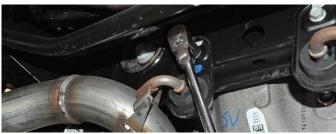
6. Use a 3/8" drive ratchet and 13mm socket, to remove the bolt holding down the driver side hanger grommet assembly.
