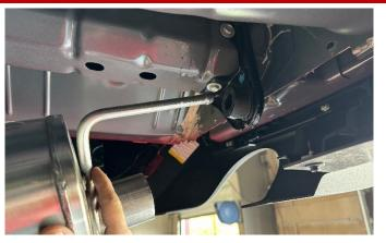
11. Slide the rear hanger into the rear hanger grommet located on the vehicle above and just inside of the passenger side tip cut out.
