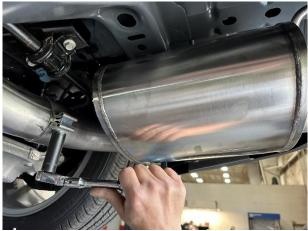
12. Slide the muffler inlet pipe over the passenger side axle pipe outlet. Tighten the clamp using the 3/8" ratchet and 15mm deep socket until the muffler assembly is snug on the axle pipe.
