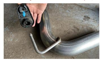
2. Locate the passenger side axle pipe assembly, and the hanger grommet assembly removed during REMOVAL STEP 11 of the stock exhaust removal process. Install the hanger grommet assembly onto the front hanger of the muffler assembly in the same position as previously installed on the stock exhaust.
