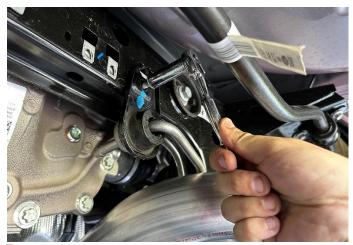
Locate a 13mm bolt set aside during REMOVAL STEP 8 of the stock exhaust removal process. Install the front passenger hanger grommet assembly onto the rear suspension sub-frame and tighten it down with the 13mm bolt, 3/8" ratchet and 13mm socket.
