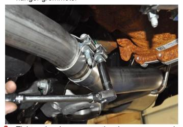
Tighten the clamp connecting the passenger axle pipe to the 3" adapter using the 3/8" ratchet and 15mm deep socket until the axle pipe assembly is snug on the adapter.
