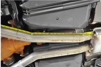
**6.** Measure 20" away from the flange on the stock resonator, following the outside profile of the exhaust pipe of the passenger side.
