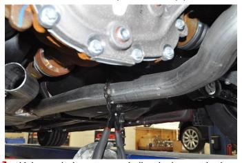
1. Using a chain cutter or similar device, cut both the driver and passenger side exhaust pipes at the marked locations. Place a jack stand or similar device under the stock tunnel section of the exhaust for support. Once the axle pipes are cut, there are no additional stock hangers supporting the tunnel section.
