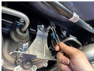
10. Locate the rear under tray mounting bracket and the two bolts set aside in REMOVAL STEP 4 of the stock exhaust removal process. Install the rear under tray mounting bracket onto the rear suspension sub-frame and tighten it down with the two bolts using a 3/8" ratchet and 13mm socket.
