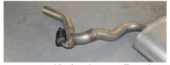
11. Remove both the driver and passenger side hanger grommet assemblies from the rear mufflers using grommet pullers or a similar device. Set aside the hanger grommet assemblies to be reused in INSTALL STEP 2.
