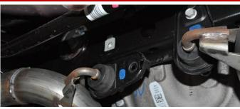
9. Once the bolt is removed, push up slightly on the exhaust and slide the hanger grommet assembly rearward to free it from the rear suspension subframe. Rotate the hanger grommet assembly a minimum of 90° so that it will not interfere with the rear suspension sub-frame.
