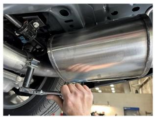
9. Slide the muffler inlet pipe over the passenger side axle pipe outlet. Tighten the clamp using the 3/8" ratchet and 15mm deep socket until the muffler assembly is snug on the axle pipe.
