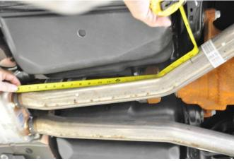
5. Starting on the driver side, measure 19 3/4" away from the flange on the stock resonator, following the outside profile of the exhaust pipe. The tape measure should follow the bend profile of the pipe.
