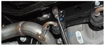
8. Using a 3/8" drive ratchet and 13mm socket, remove the bolt holding down the driver side hanger grommet assembly. Set aside the fastener in a protected location to be reused in INSTALL STEP 5.
