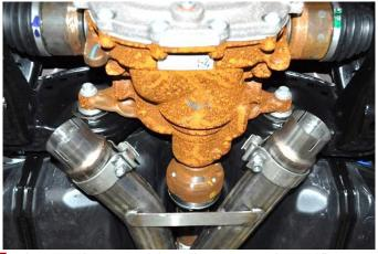
clamps. Install the clamps on the adapter so that the bolts are vertical with the nuts towards the ground and both bolts are towards the inside of the vehicle when the adapters are installed over the double H-Pipe outlets. Tighten the clamps using a ratchet and 15mm deep socket, until the adapters are snug on the pipes.
