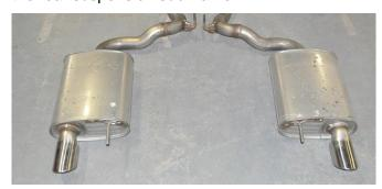
7. Lower the cut end of the driver side muffler assembly just enough to create clearance between the pipe and any suspension components. Slide the whole muffler assembly forward to remove the rear muffler hanger from the hanger grommet. The driver muffler assembly will not be free from the vehicle.
