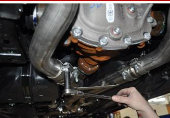
11. Repeat Install Steps 7-9 on the passenger side of the vehicle. Once the exhaust system is secure, it is safe to remove the jack stand from beneath the double H-Pipe.
