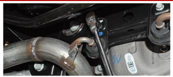
Using a 3/8" drive ratchet and 13mm socket, remove the **bolt** holding down the driver side hanger grommet assembly. Save bolt for reinstallation (Install Step 9).
