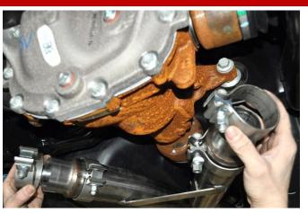
6. Locate two 2½" clamps. Install the clamps on the adapter outlet pipes so that the bolts are vertical with the nuts towards the ground and the bolts towards the outside of the vehicle. WARNING: Do NOT tighten the clamps at this step, as the stock axle pipes will then not be able to fit inside the adapters.
