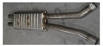
Slide the stock tunnel muffler assembly rearward to free it from the two sleeve clamps and remove it from the vehicle.
