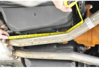
**2.** The tape measure should follow the bend profile of the pipe.
