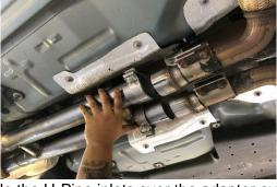
2. Install two 3" clamps on the driver and passenger inlets of the double H-Pipe so that the bolts are vertical with the nut towards the ground and the bolts towards the outside of the vehicle.
