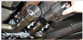
1. Locate the two inlet adapters. Slide the adapters into the factory sleeve clamps, and tighten using the ratchet and 15mm deep socket, until the adapters are snug in the clamps.
