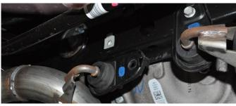
6. Once the bolt is removed, push up slightly on the exhaust and slide the hanger grommet assembly rearward to free it from the rear suspension subframe. Rotate the hanger grommet assembly a minimum of 90° so that it will not interfere with the rear suspension sub-frame.
