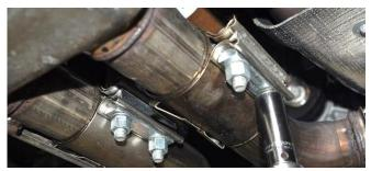
**8.** Using a 3/8" drive ratchet and 15mm deep socket, loosen the two sleeve clamps at the catback connection point. Both nuts must be loosened in order for the clamp to fully disengage.
