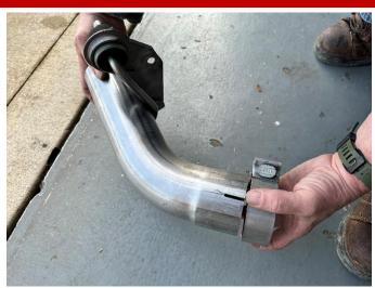
**23.** (CARBON TIPS ONLY) Locate one of the 3" clamps and slide the clamp onto the inlet of the outer tip pipe assembly. Orient the clamp so the bolt is vertical with the nut towards the ground and the bolt towards the inside of the vehicle.
