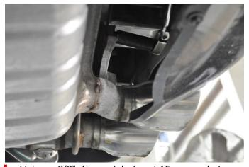
4. Using a 3/8" drive ratchet and 15mm socket, remove the two mounting nuts on each side (4 total) that hold the rear driver and passenger hanger grommet assemblies to the chassis.
