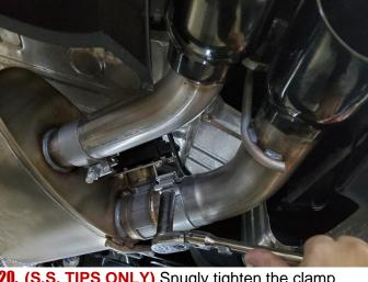
**20. (S.S. TIPS ONLY)** Snugly tighten the clamp securing the outer tip assembly to the muffler using a 15mm deep socket and 3/8" ratchet, leaving it loose enough for later adjustment.
