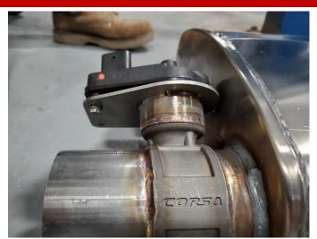
Locate the valve control unit mounting hardware from removal step 9 and start all three screws by hand.
