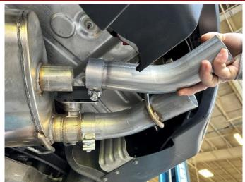
**27.** (CARBON TIPS ONLY) Slide the tip pipe assembly onto the smaller outlet of the muffler.
