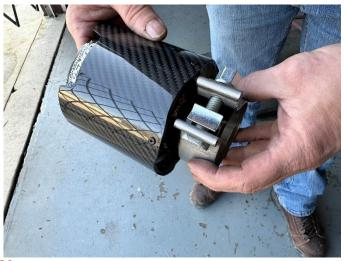
**32.** (CARBON TIPS ONLY) Locate one of the 4.5" inner carbon tip assemblies and one 2.5" clamp and slide the clamp onto the inlet of the tip assembly. Orient the clamp so the bolt is horizontal with the nut towards the inside of the vehicle.
