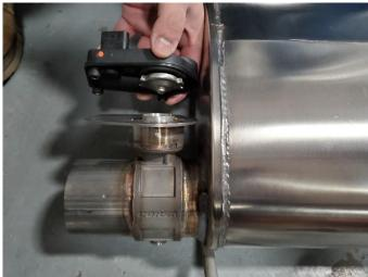
Locate the passenger muffler and the valve control unit removed from the passenger side of the stock muffler in removal step 9. Orient valve to match the rotation of the valve control unit as it was when removed from stock exhaust.
