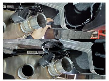
10. Route the wiring harness around the heat shield, then connect the other end of the extension to the valve control unit. Press down gray locking tab to secure. Repeat INSTALL STEPS 4-11 for the driver side muffler.
