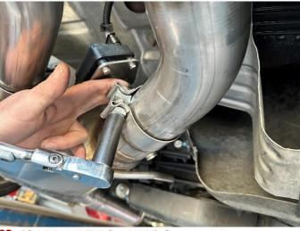
28. (CARBON TIPS ONLY) Snugly tighten the clamp securing the outer tip pipe assembly to the muffler using a 15mm deep socket and 3/8" ratchet, leaving it loose enough for later adjustment.
