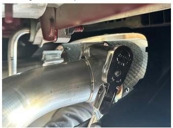
33. (CARBON TIPS ONLY) Slide the inner carbon tip assembly onto the outlet of the inner tip pipe. Snugly tighten the clamp securing the carbon tip assembly to the inner tip pipe using a 15mm deep socket and 3/8" ratchet, leaving it loose enough for later adjustment. Repeat INSTALL STEPS 30-33 for the driver side carbon tip assemblies.
