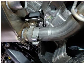
**15.** (S.S. TIPS ONLY) Slide the outer tip assembly inlet onto the valve outlet of the muffler.
