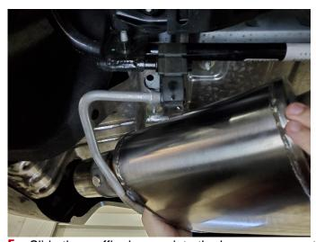
Slide the muffler hanger into the hanger grommet
