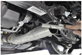
**8.** Carefully and thoroughly de-burr both stock tunnel section outlet pipes from any burrs and sharp edges. This is important, as any burrs will prevent the rear muffler inlet pipes from sliding over the stock exhaust pipes.
