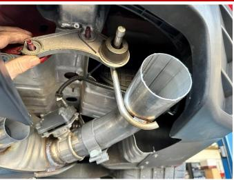
**24.** (CARBON TIPS ONLY) Install the stock hanger grommet assembly onto the mounting studs, then slide the outer tip pipe assembly inlet onto the valve outlet of the muffler.
