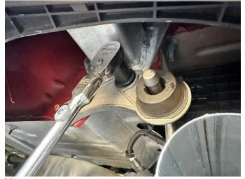
25. (CARBON TIPS ONLY) Locate the stock hanger grommet assembly mounting hardware from REMOVAL STEP 4 and start them by hand onto the mounting studs. Tighten the hanger grommet assembly hardware using a 15mm socket and 3/8" ratchet. Repeat INSTALL STEPS 22-25 for the driver side outer tip pipe assembly.
