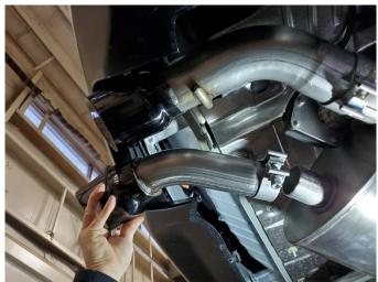
**19.** (S.S. TIPS ONLY) Slide the inner tip assembly onto the smaller outlet of the muffler.
