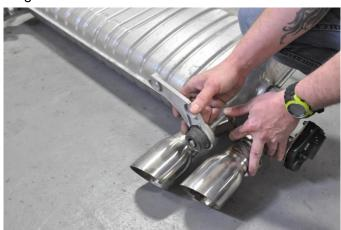
Note the orientation of each factory grommet assembly. Remove both the driver and passenger side hanger grommet assemblies from the rear mufflers using grommet pullers or a similar device.
