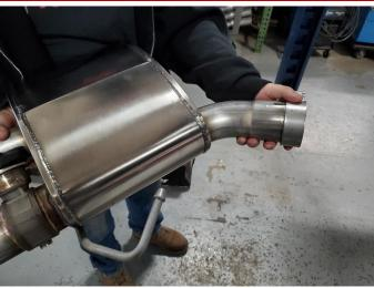
4. Locate one of the 2.75" clamps and slide over the inlet of the passenger muffler. Orient the clamp so the bolt is vertical with the nut towards the ground and the bolt towards the inside of the vehicle.
