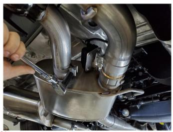
21. (S.S. TIPS ONLY) Snugly tighten the clamp securing the inner tip assembly to the muffler using a 15mm deep socket and 3/8" ratchet, leaving it loose enough for later adjustment. Repeat INSTALL STEPS 18-21 for the driver side inner tip assembly.
