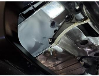
16. (S.S. TIPS ONLY) Locate the stock hanger grommet assembly mounting hardware from REMOVAL STEP 4 and start them by hand onto the mounting studs.
