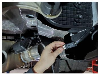
Connect the extension to the stock wiring harness. Press down gray locking tab to secure.
