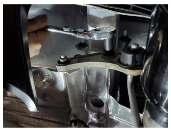
17. (S.S. TIPS ONLY) Tighten the hanger grommet assembly hardware using a 15mm socket and 3/8" ratchet. Repeat INSTALL STEPS 11-17 for the driver side outer tip assembly.
