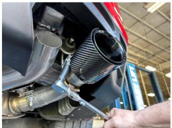
**31.** (CARBON TIPS ONLY) Slide the outer carbon tip assembly onto the outlet of the outer tip pipe. Snugly tighten the clamp securing the carbon tip assembly to the outer tip pipe using a 15mm deep socket and 3/8" ratchet, leaving it loose enough for later adjustment.
