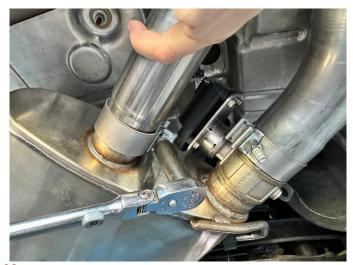
**29.** (CARBON TIPS ONLY) Snugly tighten the clamp securing the inner tip pipe assembly to the muffler using a 15mm deep socket and 3/8" ratchet, leaving it loose enough for later adjustment. Repeat INSTALL STEPS 24-29 for the driver side inner tip pipe assembly.
