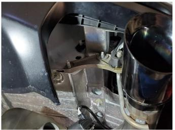
**14.** (S.S. TIPS ONLY) Install the stock hanger grommet assembly onto the mounting studs.
