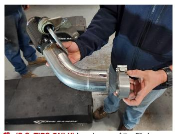
**13. (S.S. TIPS ONLY)** Locate one of the 3" clamps and slide the clamp onto the inlet of the outer tip assembly. Orient the clamp so the bolt is vertical with the nut towards the ground and the bolt towards the inside of the vehicle.
