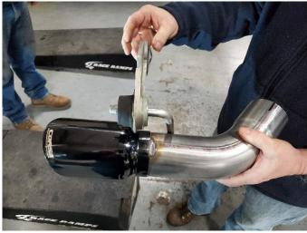
(S.S. TIPS ONLY) Install the stock hanger grommet assembly onto the tip hanger.
