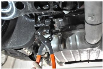
Remove the two front hangers on each side from the factory grommets using a grommet puller or similar device.
