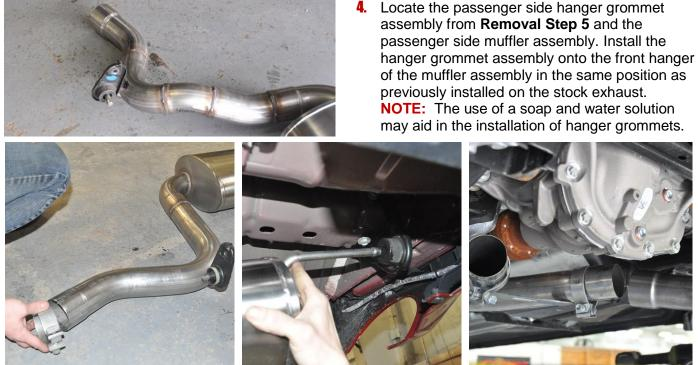
5. Locate one 3" clamp. Install the clamp on the passenger side muffler inlet pipe so that the bolt is vertical with the nut towards the ground and the bolt is towards the inside of the vehicle. Slide the rear hanger into the rear hanger grommet located on the vehicle above and just inside of the passenger side tip cut out. Slide the muffler inlet pipe over the passenger side X-Pipe outlet.
