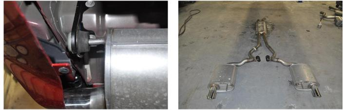
4. Slide the stock exhaust assembly rearward until the stock resonator inlet pipes are free of the sleeve clamps. Lower the front of the exhaust in order to create clearance between the resonator inlet pipes and the sleeve clamps, then slide the complete exhaust forwards to remove the rear driver and passenger side hangers from their respective hanger grommets. The stock exhaust assembly will now be free from the vehicle.
