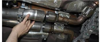
3. Slide the X-Pipe inlets over the X-Pipe adapter outlets. Position the X-Pipe so that the cross-brace located at the rear of the X-Pipe is facing down and is parallel with the ground, and the outlets are centered around the rear differential. Tighten the clamps using a ratchet and 15mm deep socket until the X-Pipe is snug on the adapters. Place a jack stand or similar device under the X-Pipe for support.
