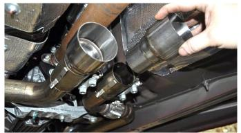
1. Locate the two X-Pipe inlet adapters. Slide the adapters into the factory sleeve clamps, and tighten the clamps using a ratchet and 15mm deep socket, until the adapters are snug in the clamps.
