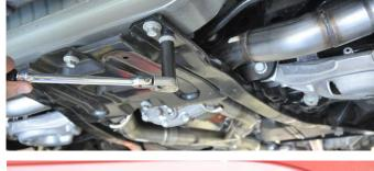
Locate the passenger side convertible brace and hardware from **Removal Step 1.** Slide the front of the brace over the front bolt then install the furthest rear bolt to support the brace. Using a 3/8" drive ratchet and 13mm deep socket install the remaining bolts. Repeat this procedure for the driver side brace. Tighten all bolts supporting the factory brace to manufacture specifications.
