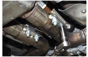
Using a 3/8" drive ratchet and 15mm deep socket, loosen the two sleeve clamps at the catback connection point. Both nuts must be loosened in order for the clamp to fully disengage.
