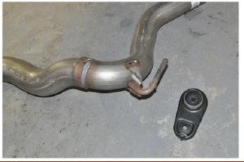
Remove both the driver and passenger side hanger grommet assemblies from the front muffler hangers using grommet pullers or a similar device. Save both grommets for reinstallation (Install Step 4).
