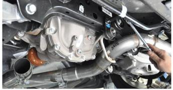
6. Locate the 13mm bolt from Removal Step 3. Install the front passenger hanger grommet assembly onto the rear suspension sub-frame and tighten it down with the 13mm bolt, using the 3/8" ratchet and 13mm socket.
