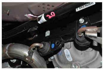
Using the 3/8" drive ratchet and 13mm socket, remove the bolt holding down the driver side hanger grommet assembly. Once the bolt is removed, push up slightly on the exhaust and slide the hanger grommet assembly rearward to free it from the rear suspension sub-frame. Rotate the hanger grommet assembly a minimum of 90° so that it will not interfere with the rear suspension sub-frame. Save bolt for reinstallation (Install Step 6). Repeat this process for the passenger side hanger grommet assembly.
