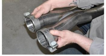
Locate the Double X-Pipe and two 3" clamps. Install the clamps on the driver and passenger X-Pipe inlets so that the bolt is vertical with the nut towards the ground and the bolts towards the outside of the vehicle.
