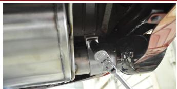
9. Locate the passenger rear tip assembly and one 3" clamp. Install the clamp on the tip inlet pipe so that the bolt is horizontal with the nut towards the inside of the vehicle and the bolt towards the top. Slide the tip assembly over the muffler outlet pipe and tighten the clamp using the ratchet and 15mm deep socket until the tip assembly is snug on the muffler outlet pipe. Repeat this process for the driver side.
