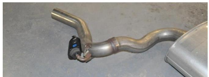
**IMPORTANT:** Carefully and thoroughly de-burr the stock tunnel muffler (resonator) outlet pipes from any burrs and sharp edges. This is important as any burrs will prevent the stock to axle-back adapters from sliding over the stock exhaust pipes. This concludes the factory exhaust system removal.
