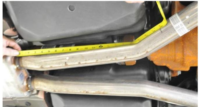
2. On the driver side, measure 19 3/4" away from the flange on the stock resonator, following the outside profile of the exhaust pipe. The tape measure should follow the bend profile of the pipe.
