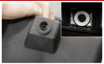
Locate the CORSA air box, and the factory grommet and metal bushing from Removal Step 7 and install grommet in air box then the metal bushing into grommet from inside box.
