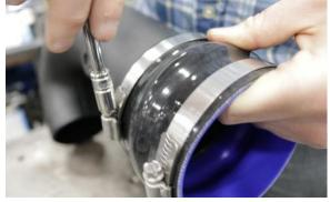
10. Locate the hump hose and two # 64 clamps. Install the hump hose and one clamp onto the air duct inlet end and tighten clamp using a flathead screwdriver or ratchet and 8mm socket. Loosely place other clamp on hump hose.
