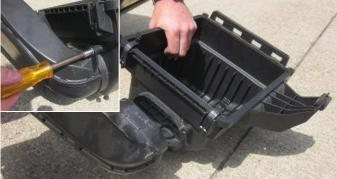
8. Remove the bolt attaching the scoop to factory air box using a ratchet and 8mm socket. Remove the factory air scoop from the bottom of the air box
