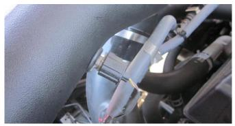
**16.** Clip wiring harness on air temperature sensor.
