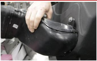
2. Locate the 6mm x 25mm bolt, .25" x .75" flat washer, one .25" x .63" flat washer, one .25" lock washer, 6mm nut, .25" spacer, and factory air scoop from removal step 8. Attach air scoop to air box placing the spacer between the scoop tab and air box. Tighten hardware with 10mm wrenches.
