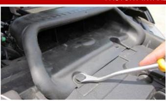
Remove the two plastic clips from the factory air scoop using a trim removal tool.
