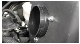
**8.** Locate three 6mm x 16mm bolts, three .25" x .63" flat washers, and three .25" lock washers. Attach filter adapter to air box and tighten using a ratchet and 10mm socket.
