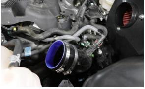
11. Locate straight sleeve and remaining two #64 clamps. Install straight sleeve and one #64 clamp onto driver side turbo inlet tube and tighten clamp using a flathead screwdriver or ratchet and 8mm socket. Loosely place other #64 clamp onto straight sleeve.
