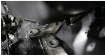
Install CORSA air box into the vehicle by inserting posts on bottom of CORSA air box into factory grommets.
