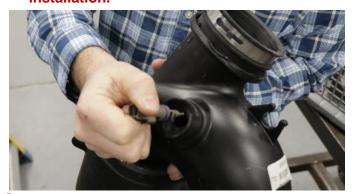
9. Remove the air temp sensor from factory duct by gently lifting tab and rotating counterclockwise until it stops then pulling straight out. NOTE: Save for installation.
