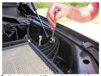
Use a ratchet and 13mm socket or wrench to remove the bolt holding the air box to the vehicle.
