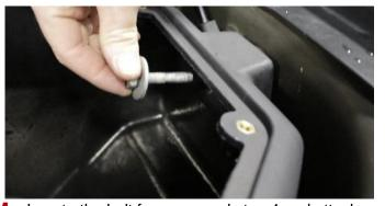
4. Locate the bolt from removal step 4 and attach the CORSA air box to the inner fender using a ratchet and 13mm socket.
