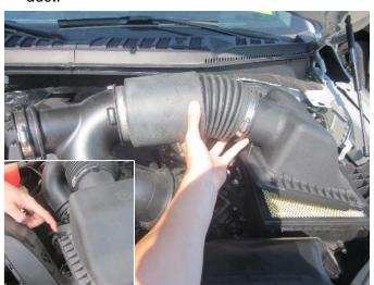
**3.** Unclip the air box lid and remove the factory duct and lid assembly as one piece.
