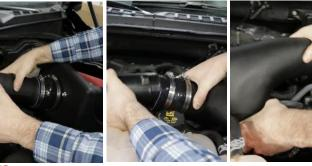
13. Install air duct into vehicle by placing the hump hose onto the filter adapter, then place reducer onto the upper stock inlet. Rotate duct down and into the straight sleeve.
