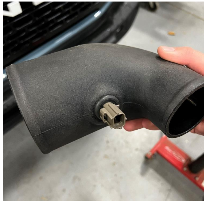
4. Install the temperature sensor to the air duct by fitting it through the rubber grommet. Make sure the sensor is oriented as shown.
