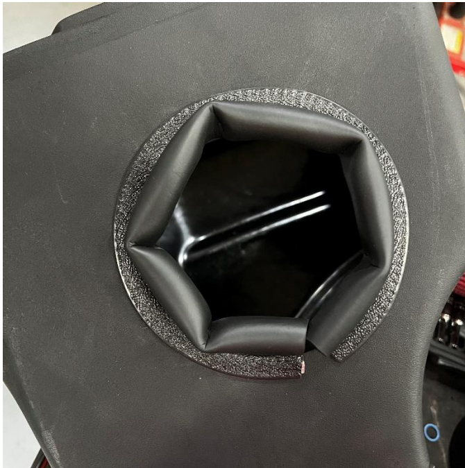
1. Install filter bulb seal trim onto the CORSA air box.
