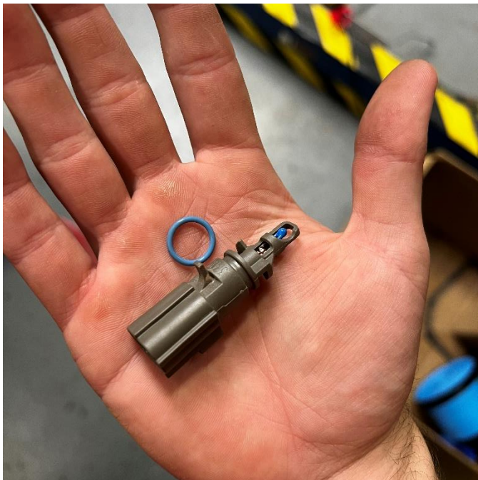
3. Remove the O-ring from the temperature sensor.
