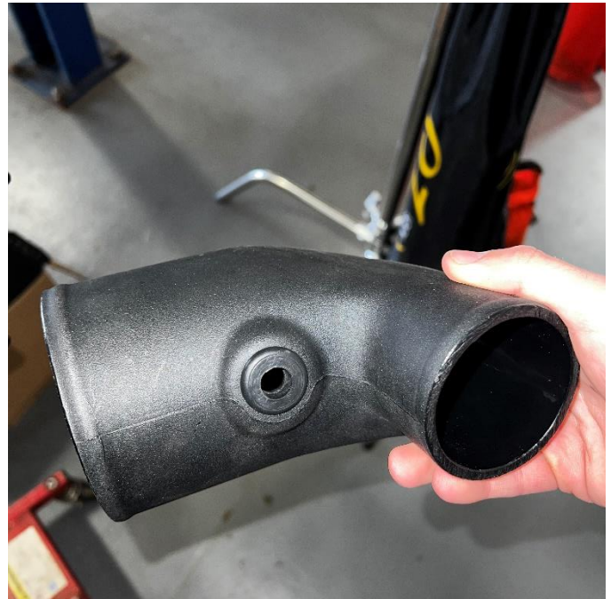
2. Install the rubber grommet into the CORSA air duct.
