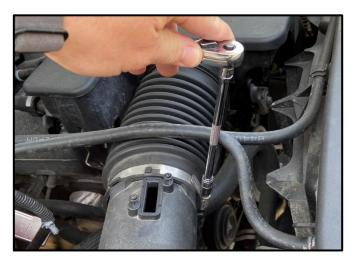
Using an 8mm Socket & Ratchet or Wrench, loosen the Hose Clamp connecting the Factory Air Duct to the Factory Air Box. This will not be reused.
