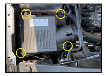
**9.** Using an 8mm Socket & Ratchet or Wrench, remove the 4 bolts holding the Factory Air Box Lid from the Base. These will not be reused.
