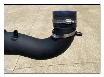
5. Locate the CORSA Air Intake Duct, the 2 Hose Clamps, the 2 Thread to Barb Fittings and either the Ø4in to Ø3.5in Reducer (6.2L) or Ø3.5in Hose (5.3L) (shown). Assemble the parts to the Air Intake Duct as shown. The Thread to Barb Fittings should be tightened until they are tight and flush to the mating surface on the Air Intake Duct. The hose clamps should be loose at this time.
