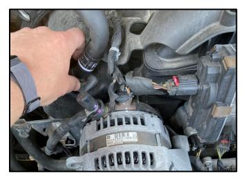
**8.** After the Factory Air Duct is removed, go back to the Factory Hoses. Squeeze the Grey Tabs, pull up and remove the hoses. These will not be reused.
