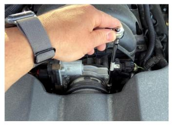
5. Using an 8mm Socket & Ratchet or Wrench, loosen the Hose Clamp connecting the Factory Air Duct to the Throttle Body. This will not be reused
