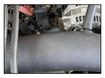
Locate the MAF Sensor Gasket and install it onto the MAF Senor removed in from Removal Step 3. Next, slide the MAF Sensor and Gasket into the opening in the back of the Air Intake Duct. The Flat Side goes up and the screws will only align one way. Then locate MAF Screws from the Hardware Kit and use a Phillips Screwdriver to secure the MAF Sensor to the Air Intake Duct. Once the MAF Sensor is secured, reconnect the Wire Harness and push the Red Locking tab down.
