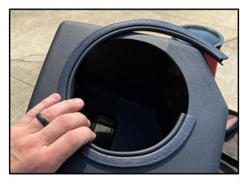
1. Locate the CORSA Air Intake Box and the Box Opening Seal. Starting on the bottom of the opening, press the Seal around the opening.
