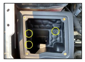
3. Align the Mounting Slots in the bottom of the Air Intake Box to the Factory Mounts. Then, locate the bolts for the Factory Air Box Mounting Tray in Removal Step 11. Hand thread 3 of the Bolts into the Factory Mounts. Make sure the Air Intake Box is close as you can get it to the Fender.
