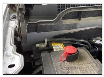
**15.** Use a 10mm Socket & Ratchet or Wrench to reconnect and tighten the negative battery terminal.
