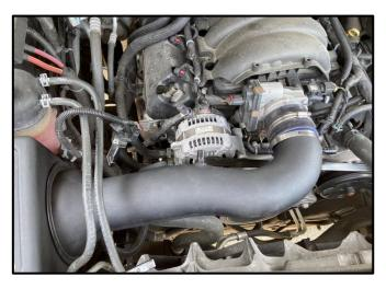
6. Next, install the assembled Air Intake Duct into the vehicle. Begin by sliding the large end into the opening in the Air Intake Box. Next, rotate and move the Air Intake Duct until the Hose or Reducer are aligned with the Throttle Body. Then slide the Hose or Reducer on to the Throttle Body and arrange the Hose Clamps as shown. On the 6.2L, the larger clamp goes on to the Throttle Body. Once everything is properly aligned, use an 8mm Socket & Ratchet or Wrench to secure the Hose Clamps.
