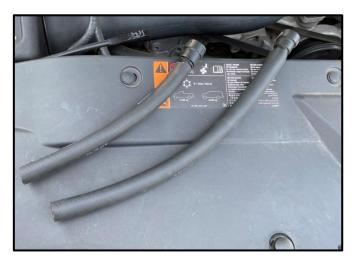
1. Locate the 2 Hoses and 2 Quick Connect Fittings. Press the fittings into one end of the hoses, as shown.
