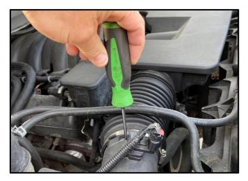
3. Using a T15 Torx Driver, remove the Factory MAF Screws. These will not be reused. Next, disconnect the Mass Air Flow (MAF) Sensor from the Wire Harness by pulling the red clip up and then squeeze the sides of the Wire Conncetor to release it. Carefully remove the MAF Sensor and store it in a safe location. It will be reused in Installation Step 9.
