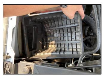
10. Lift the Factory Air Box Lid from the Factory Air Box Base. To remove the Base, lift the right side up to release it from the Grommets, and then pull the Base toward the engine to release the base from the Fender. This will not be reused.
