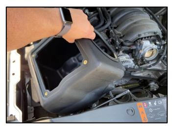
After the Seal is installed, install the Air Intake Box into the vehicle. This is done by sliding the Side Inlet Duct through the opening in the Fender and the Lower Inlet Scoop through the opening above the fender.
