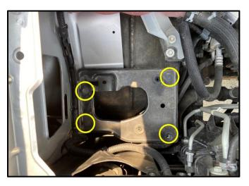
11. Using a 10mm Socket & Ratchet or Wrench, remove the 4 bolts holding the Factory Air Box Tray from the Vehicle. Store them in a safe location. 3 of the 4 screws will be reused in Installation Step 3.
