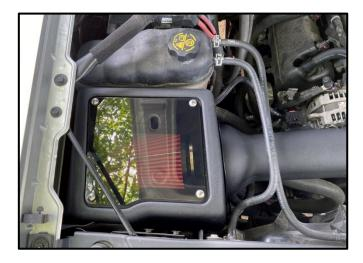
14. Using a Phillips Head Screwdriver, install the CORSA Intake Lid. Start by loosely installing the upper left screw (round hole) first. The other 3 screws are in a curved slot to help with alignment.
