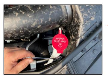
**16.** Locate the Screw from Removal Step 11. Align the Screw and Hole in the Heat Shield Mounting Tab with the threaded hole in the Vehicle. Using a 10mm Socket & Ratchet or Wrench, push down firmly on the Heat Shield so it is as low as it can be and tighten the screw.
