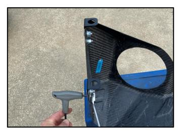
Locate the CORSA Carbon Fiber Heat Shield, 2 90deg Brackets, and M8 Hardware. Use a 5mm Hex Driver and 13mm Socket & Ratchet or Wrench to tighten the Hardware.
