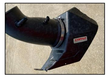
Locate 6.50in T-Bolt Clamp. Remove the Nut from the T-Bolt Clamp. Open the T-Bolt Clamp and wrap it around the open end of the Air Filter. Next, close the T-Bolt Clamp and thread the Nut back onto the Stud of the T-Bolt Clamp. Snug the T-Bolt Clamp with a 10mm Socket & Ratchet or Wrench, securing the Duct and Filter.
