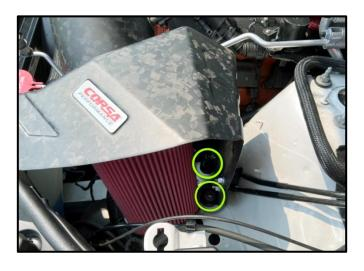
14. Install the CORSA Duct, Filter, and Heat Shield into the vehicle. Insert the Duct into the Angled Reducer first. Next, rotate the Heat Shield and Duct into position and align the Factory Grommets with the Mounting Studs on the Inner Fender area. Ensure the front tab of Heat Shield goes in front of the Washer Fluid Reservoir.
