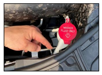
**17.** Locate the Push Rivet for the Washer Fluid Reservoir, from Removal Step 10. Rotate the Washer Fluid Reservoir back into position and reinstall the Push Rivet.
