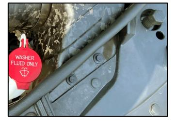
**18.** On the Hood Seal, locate the Green Pin from Removal Step 9. Insert the Push Pin into the Hole in the Heat Shield.
