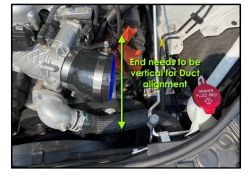
6. Locate the 4.0in to 4.5in Angled Reducer, 4.375in T-Bolt Clamp, and 4.75in T-Bolt Clamp. Assemble the 4.375in T-Bolt Clamp over the smaller end of the Angled Reducer and the 4.75in T-Bolt Clamp over the larger end. Rotate the Angled Reducer so the larger end is vertical. Snug the smaller T-Bolt Clamp with a 10mm Socket & Ratchet or Wrench but do not fully tighten at this time. Leave the large T-Bolt Clamp loose at this time.
