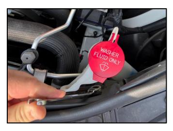
**11.** Gently push the Washer Fluid Reserviour toward the engine to reveal the Screw in front of it. Use a 10mm Socket & Ratchet or Wrench to remove the Screw and store it in a safe location. It will be reused in Installation Step 17.
