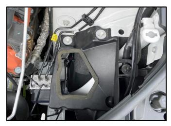
**1.** After removing the Factory Air Box, remove the Factory Mounting Bracket. This will not be reused.
