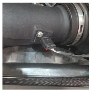
**12.** Plug MAF sensor wiring harness into sensor. Press red locking tab in to secure.
