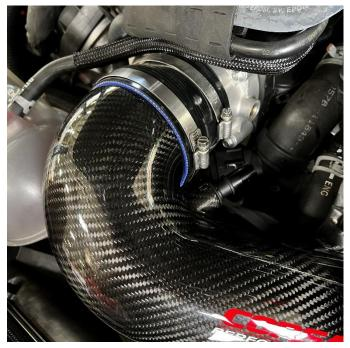
8. Attach the reducer sleeve on to the throttle body.
