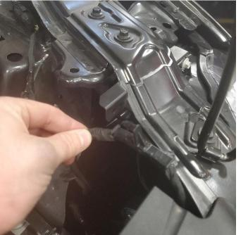
**17.** Unclip MAF wiring harness.
