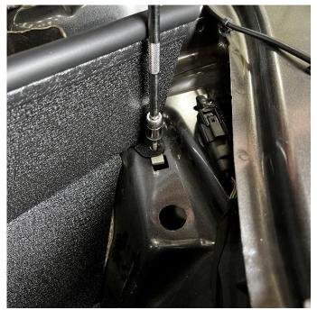
**1.** Use the 10mm bolt that was removed in removal step 14 to secure the shield.
