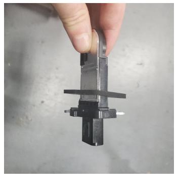
**3.** Place the included MAF gasket onto the MAF sensor.
