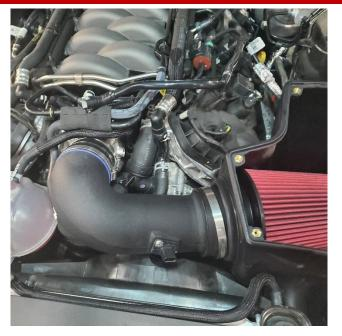
Install filter band clamp onto filter. Install air duct into position in vehicle with #56 clamp on smaller end of reducer pushing reducer onto throttle body until seated. Tighten all three clamps using 8mm socket.
