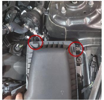
**11.** Undo two clips securing the upper airbox to the lower half.
