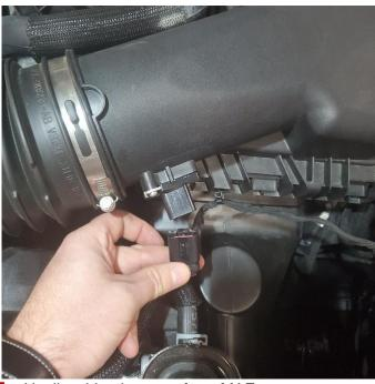
4. Unclip wiring harness from MAF sensor.
