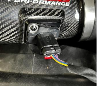
**10.** Clip MAF sensor wiring harness back into the MAF sensor in the correct orientation
