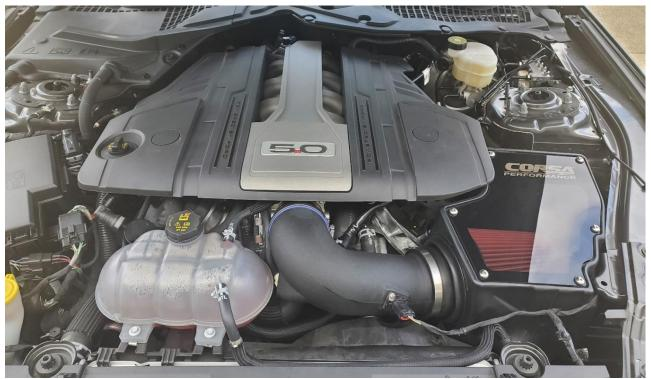
14. Install engine cover re-using factory hardware.
