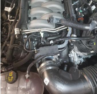
**10.** Pull duct from throttle body.
