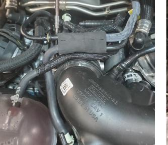
9. Using 7 mm socket loosen throttle body clamp.
