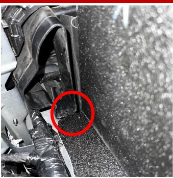
6. Insert the shield into the engine bay. The tab on the end of the shield will sit on top of the inlet tube.
