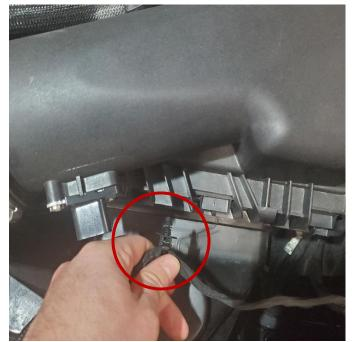
**5.** Pull wiring harness retention clip from air box.
