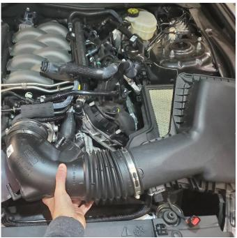
**12.** Remove duct with upper airbox.
