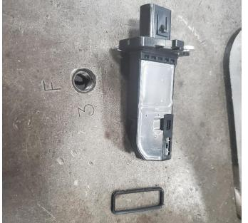
19. Remove gasket from sensor. <u>IMPORTANT:</u> KEEP GASKET ON SENSOR IF YOU HAVE CORSA'S CARBON FIBER AIR DUCT.
