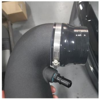
8. Install silicone reducer onto CORSA air duct along with #64 clamp.
