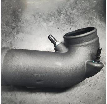
Install large fitting in threaded hole on inside of bend (left fitting in picture). Install small fitting in threaded hole on outside of bend (right fitting in picture). Tighten fittings until completely seated but do not overtighten.
