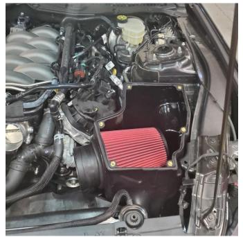
Install bulb seal trim around filter opening, then install filter into air box and through opening. Removing the filter band clamp will help with installation of filter.
