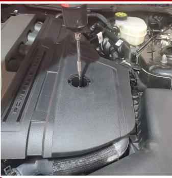
**2.** Using a 10mm socket remove the two nuts securing the engine cover.
