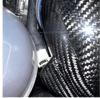
**12.** Re-attach the breather line to the smaller quick disconnect fitting.
