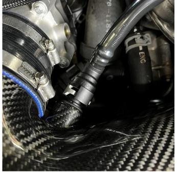
**11.** Re-attach the breather line to the larger quick disconnect fitting.
