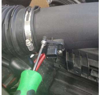
**18.** Remove MAF sensor from factory duct with T20 Torx driver.
