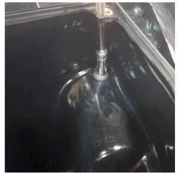
**6.** Secure CORSA air box using bolt from Removal Step 14 and 10mm socket.
