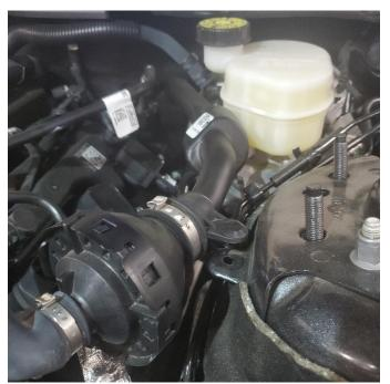
**15.** Unclip sound tube from shock tower
