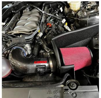
**9.** Attach the filter to the opposite end of the duct and tighten all clamps using an 8mm socket.
