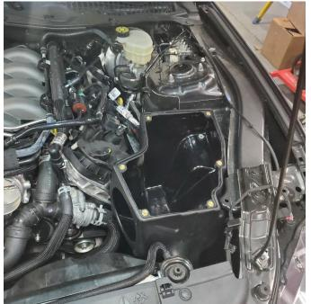
**5.** Install CORSA air box into position in vehicle. Ensure front scoop installs over factory inlet.
