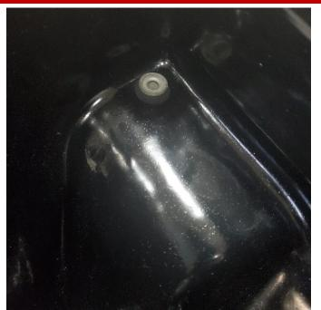
1. Insert grommet and bushing from removal step 20 into CORSA air box.
