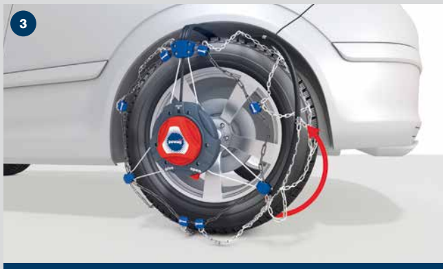
Demounting pewag servomatik
