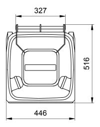
Waste Recycling Bins MGB 60 Litre Sizes, Measures, Dimensions: Hight 935 mm; Width 445 mm; Depth 520 mm
