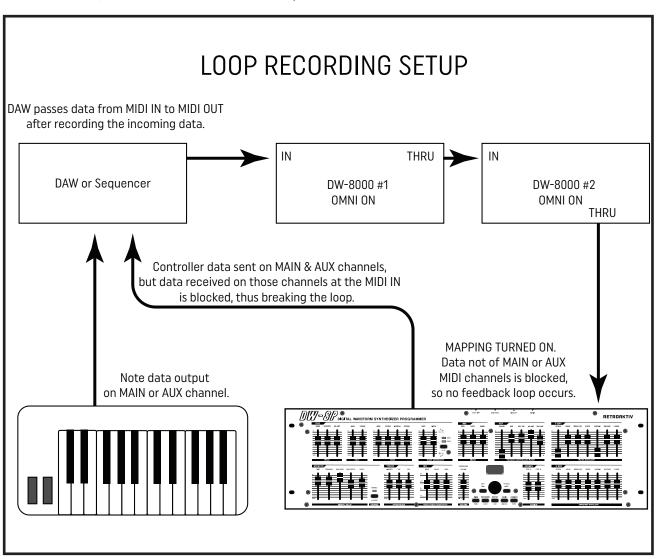
An alternate method of loop recording is shown below. This method bypasses the controller's merging function, and eliminates any latency from the controller. The latency from the controller is only noticeable if you are sending large amounts of CC, SYSEX, and NOTE data at once. Using this method will allow the fastest note and data processing time. Be sure to either turn FILTER on or use the MAP function, so a feedback loop is not introduced.
