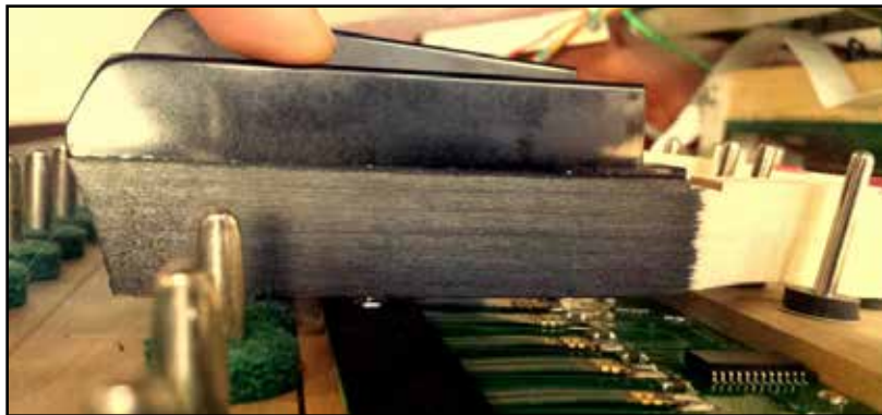
Figure 23 - Black Key Depressed (No Aftertouch Engaged)
