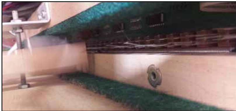
Figure 26 - Back of Key Hitting Back Rail Felt During Keystroke
