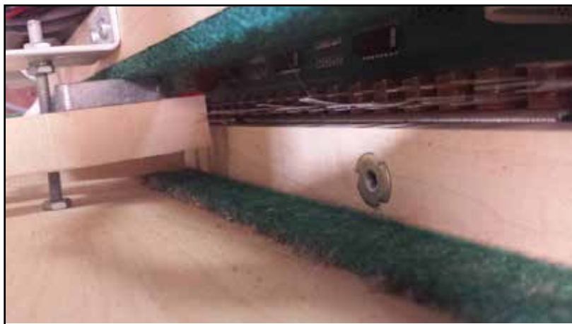
Figure 27 - Back of Key Pressing on Back Rail When Aftertouch is Engaged
