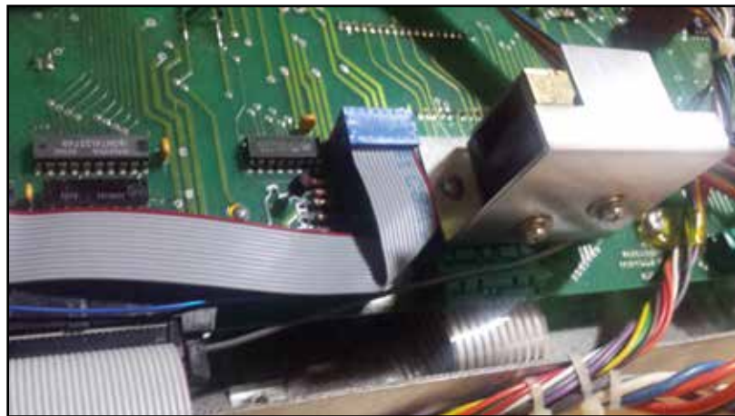
Figure 11 - 14 Pin DIP Cable Plugged Into Chroma I/O PCB J22 (Note pin number markings on PCB and Header)
