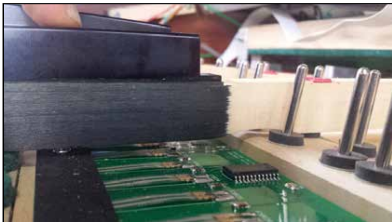
Figure 24 - Black Key Depressed (Aftertouch Engaged)
