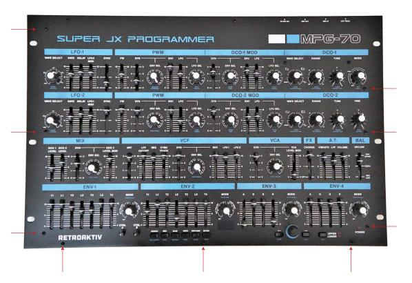
Use the diagram above to locate the 9 front panel screws to be removed. Do not remove any of the screws not marked with arrows, as this will create mor work for you and make reassembly more difficult. The 4 screws that are not removed are the ones holding the rear plate to the face. The face and rear plate are removed as one assembly.
