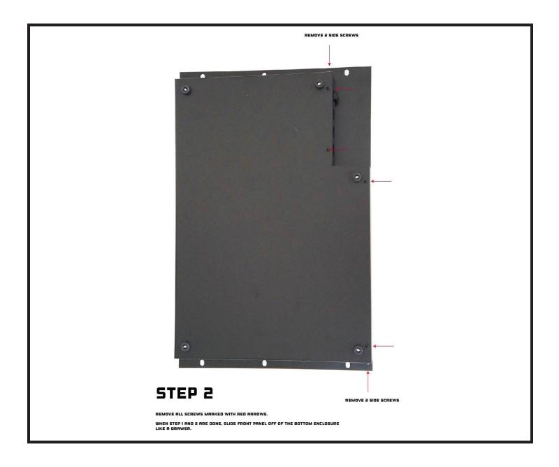
Now that the screws have all been removed, the faceplate can be removed from the rear enclosure by sliding the face toward the back of the unit.
