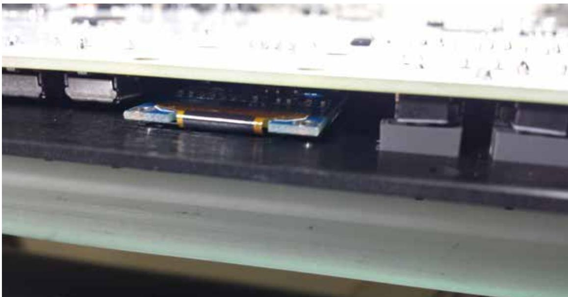
Finally, test the movement of the 2 tall trimmers. They should be easy to move. If they are not, adjust their positioning so they are not chafing the panel and they move freely. Solder into place.
