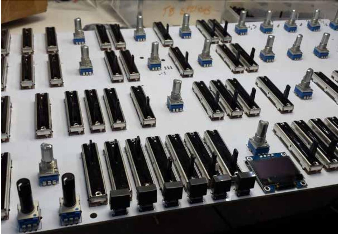
Now lower the front panel onto the PCB. Take care to make sure that the switches and pots that aren't yet soldered do not get pulled from their holes. When the panel falls into place, use the nylon nuts to hold the PCB to the protruding 5 screws under the board.
