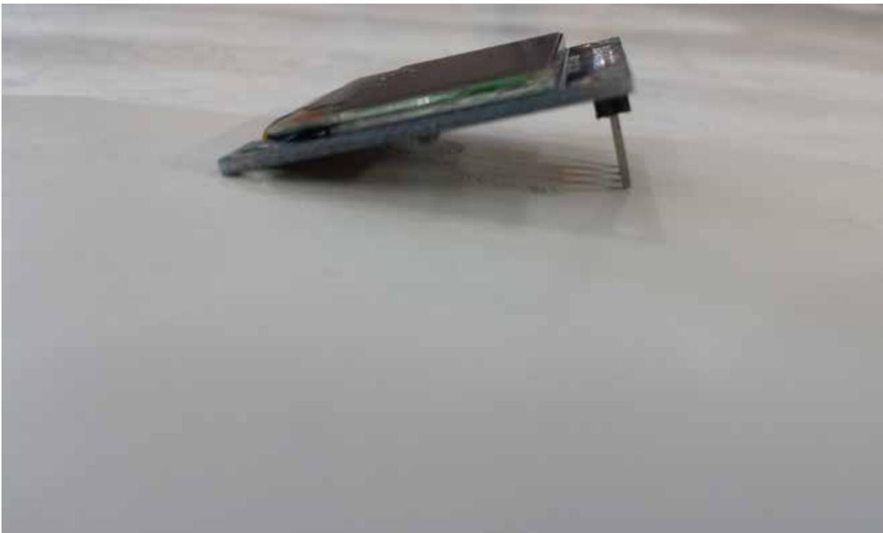
Now place the screen, the encoder, and the LED. (The short lead of the LED goes into the square hole) Do not solder yet. Just fit them in their respective holes. Attach the switch caps to their respective switches.
