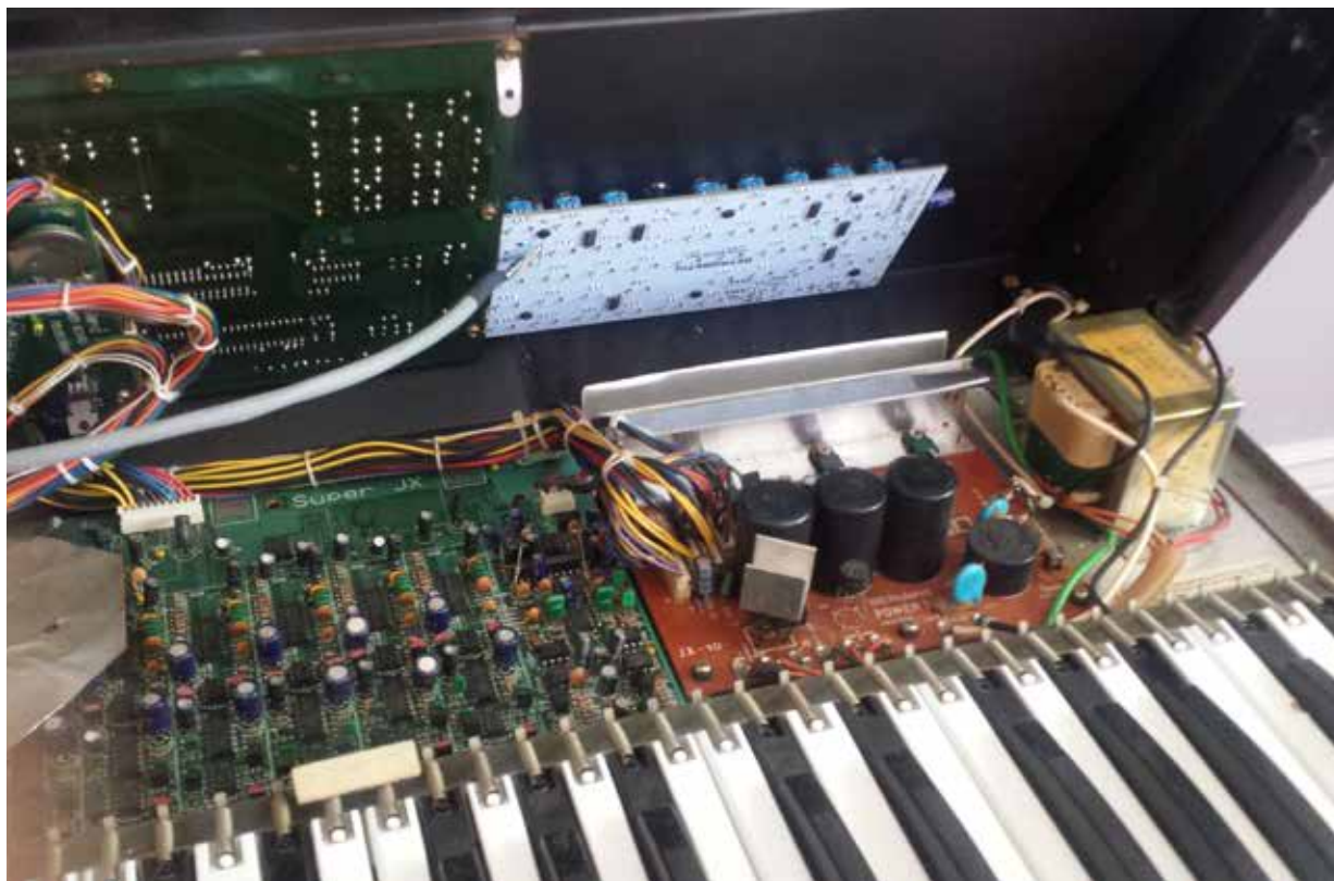
Figure 6 - Super JX with heat sink modified. (L shape bent into fin, and rear fin trimmed by 10mm)
