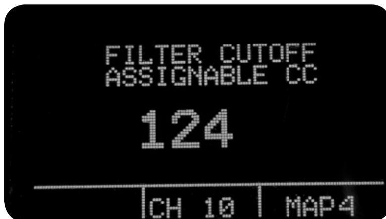
in the MIDI PROTOCOL menu. To view or "peek" at a slider's CC assignment, navigate to the MAIN MENU screen and press ENTER.
