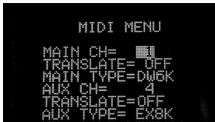
and AUX channels are set to different values. The DW-8P will not transmit sysex if both channels are set to the same value.
