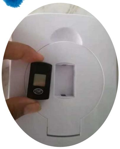
Take the new indicator and install the indicator as the picture(note the direction)
