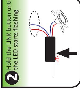
**2** Hold the LINK button until the LED starts flashing
