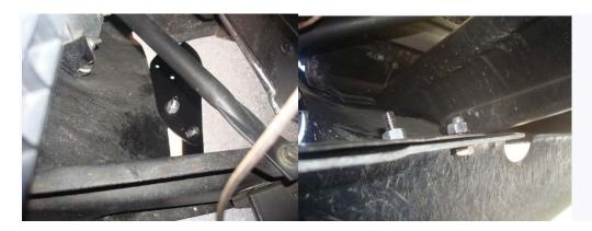
5. After making sure both brackets have the correct angle and the spoiler fits nice against the brackets, you can mark and drill the hole in the spoiler to mount the outer ends to the end brackets. We only used one bolt on each end but you can use two if desired. NOTE: Make sure that the spoiler is not actually touching the bumper at the outer ends...it will be close but not touching. (see pics)
