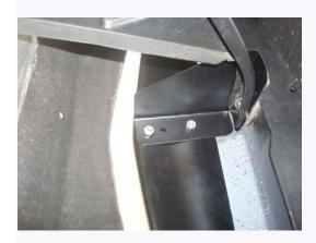
3. Find the center of the spoiler and line it up as desired with the hole in the center bracket. Mark and drill the first hole in the spoiler to mount it to the bracket with one nut, bolt and a washer on the underside of the spoiler. The center of the spoiler should be about ½ to ¾ inch away from the bumper.
