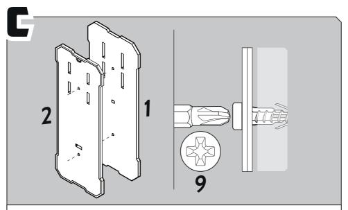
Put part 1 & 2 together and screw into the wall using marking made step B. Do not overtighten screws to avoid cracking of the acrylic.
