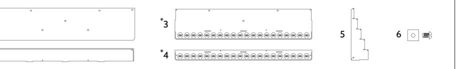
\*While the process remains the same, some parts found in LDS902.3.3 and LDS902.5.3 are different widths, therefore requiring additional screws. LDS902.3.3 requires x9 cubes and scews. LDS902.5.3 requires x11 cubes and screw.
