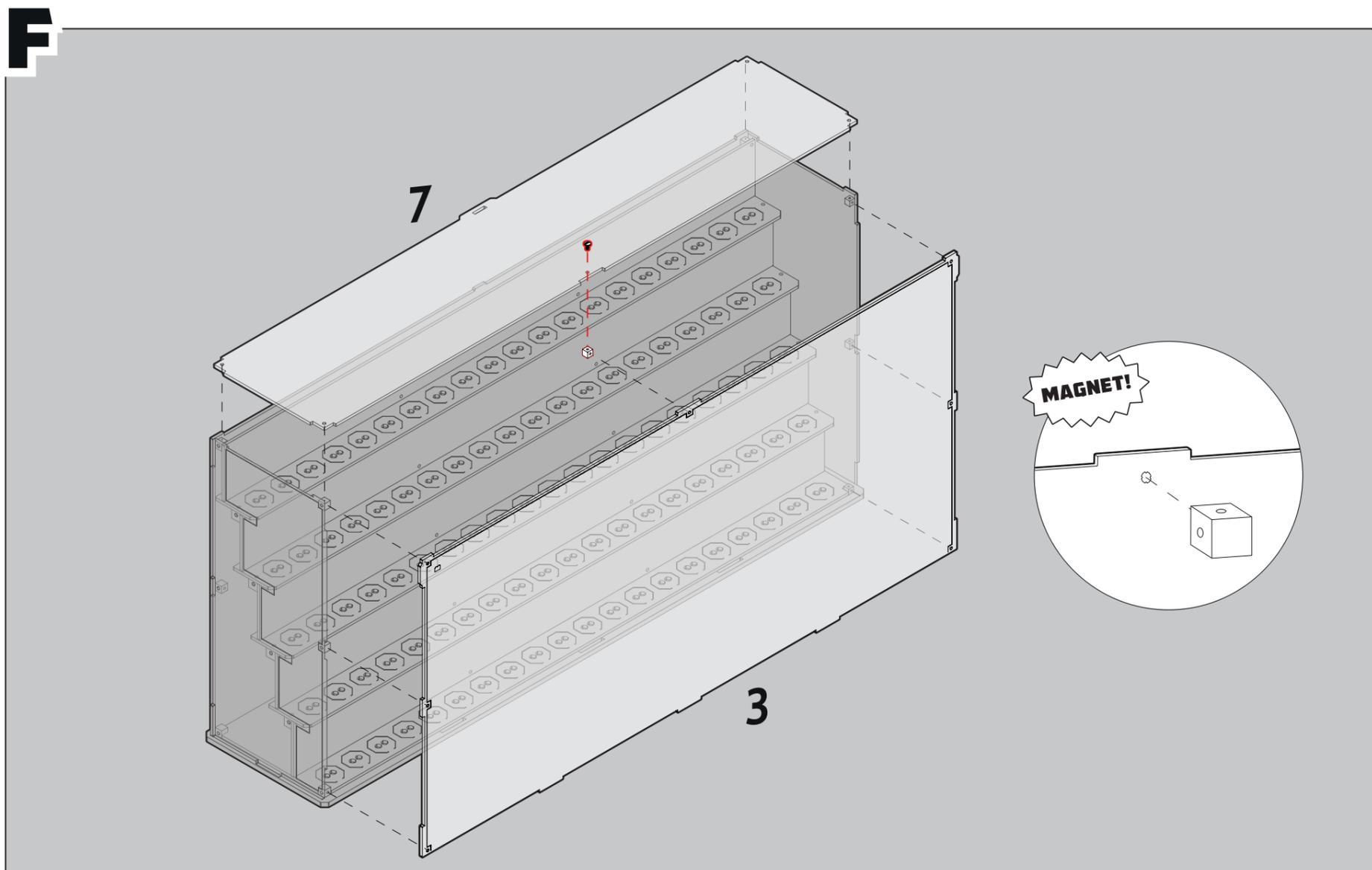
Attach part 3 onto the front of the case before attaching part 7. The areas highlighted in red require screws when connecting the cubes. The remaining cubes are connected via magnets already in parts 3 & 7.
