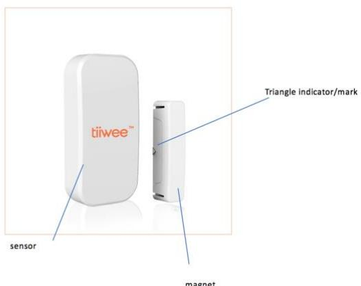
The Door & window sensor consists of a magnet and a sensor which contains a detector for changes in magnetic fields ('flux'). When the magnet is moved away from the sensor, the detector will detect that motion and will send a wireless signal to the Tiiwee A1- or A2 Alarm unit. The Tiiwee Alarm unit will now emit a strong alarm sound or a Chime depending on the settings of the Alarm unit.
