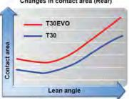
New rear profile improves contact charactoristics at higher camber angle. Larger contact area for greater grip in mid-to high-angle leans.
