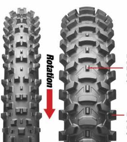
Low height of small centre block for mud releasing characteristics.
