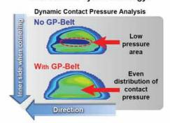
Grooves are aligned in the direction of the forces when cornering for greater stability, block stiffness & consistency. Parallel grooves along center strip. for better water channeling.
