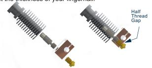
This tightening of nozzle when hot is important. It helps prevent plastic leaking out from heater block. If you tighten nozzle when cold, then heat block, the seal between threaded tube and brass nozzle will spread apart. Tightening must occur when block is hot. Please heat block before when loosening nozzle for replacement. Plastic will work as a glue, unless it is heated. Be careful. It's HOT! :)
